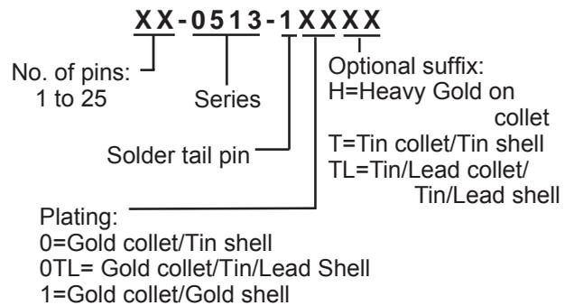
Pin-Line collet sockets also available with wire wrap pins. Consult Data Sheet No. 12014.
