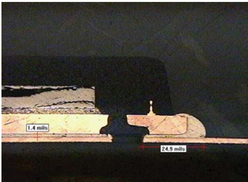
37% Paste Coverage, Plugged Via, 1.4 mil Standoff
