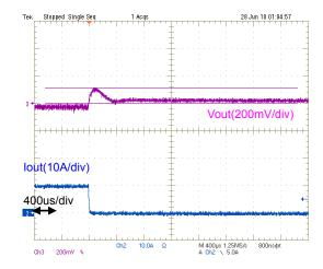
Fig.9-2-12. Load Transient Response (Io=10A  $\rightarrow$  0A)
