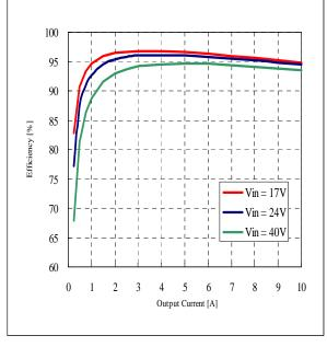
Fig.9-1-2. Efficiency v.s. Output Current
