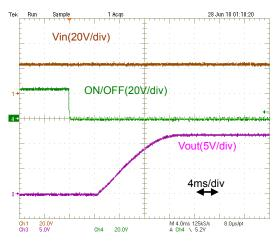
Fig.9-2-9. Start-up Waveform(Io=0A)
