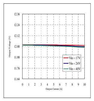
Fig.9-1-4. Output Voltage v.s. Output Current
