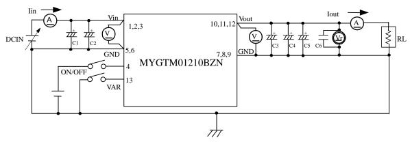
C1,C2 : 1000µF/50V Low Impedance Aluminum Electrolytic Capacitor(ZL series : Rubycon)
