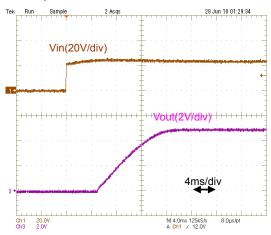
Fig.9-2-1. Start-up Waveform(Io=0A)
