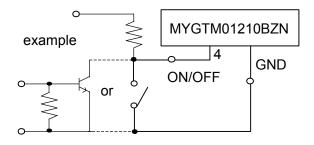
ON/OFF pin is pulled down inside of the DC-DC converter, so voltage appears up to GND at ON/OFF pin.
