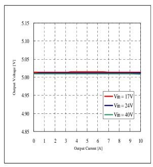
Fig.9-1-1. Output Voltage v.s. Output Current
