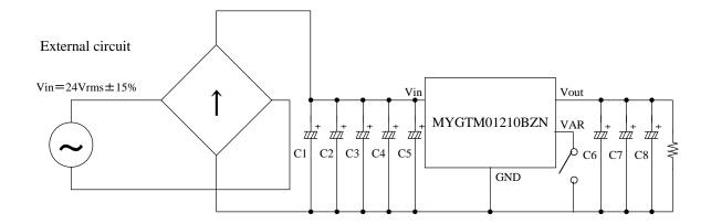
C1,C2,C3: 1000μF/50V Low Impedance Aluminum Electrolytic Capacitor (EKZE500EC3102ML25S C4,C5 NIPPON CHEMI-CON)
