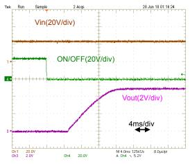
Fig.9-2-3. Start-up Waveform(Io=0A)
