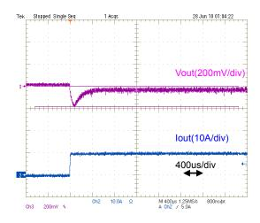
Fig.9-2-11. Load Transient Response ( $lo=0 \rightarrow 10A$ )
