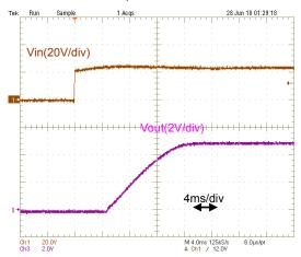
Fig.9-2-2. Start-up Waveform(Io=10A)
