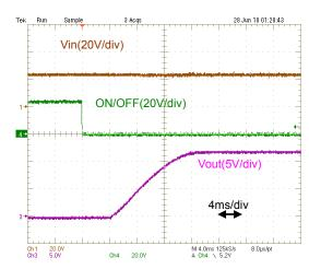
Fig.9-2-10. Start-up Waveform(Io=10A)
