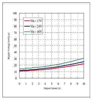
Fig.9-1-3. Ripple Voltage v.s. Output Current
