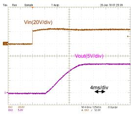
Fig.9-2-7. Start-up Waveform(Io=0A)
