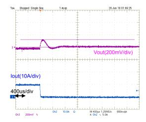
Fig.9-2-6. Load Transient Response (Io=10A  $\rightarrow$  0A)
