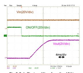
Fig.9-2-4. Start-up Waveform(Io=10A)
