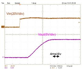
Fig.9-2-8. Start-up Waveform(Io=10A)
