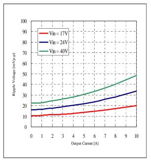
Fig.9-1-6. Ripple Voltage v.s. Output Current
