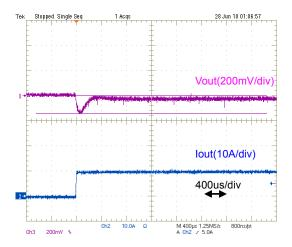
Fig.9-2-5. Load Transient Response (Io=0  $\rightarrow$  10A)
