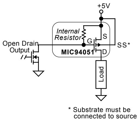
**Figure 2. Load Switch Application
