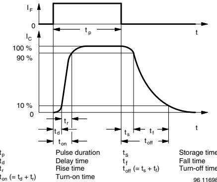
Fig. 3 - Switching Times
