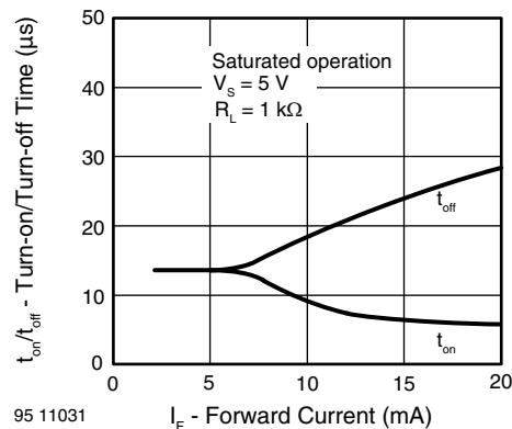
Fig. 12 - Turn-on/Turn-off Time vs. Forward Current
