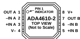
Figure 5. ADA4610-2 Pin Configuration, 8-Lead LFCSP_VD (CP Suffix)
