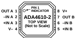
Figure 5. ADA4610-2 Pin Configuration, 8-Lead LFCSP_VD (CP Suffix)
