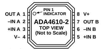
Figure 5. ADA4610-2 Pin Configuration, 8-Lead LFCSP_VD (CP Suffix)
