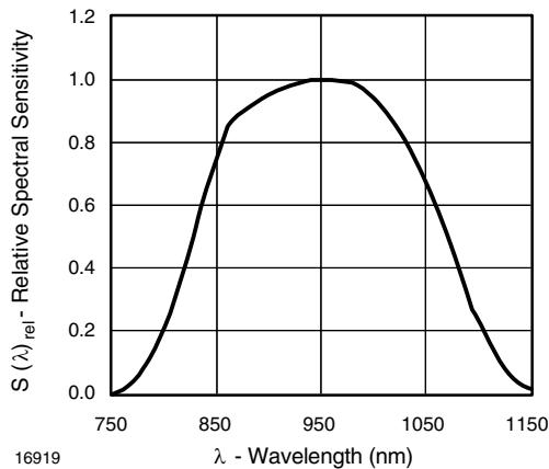
Fig. 11 - Relative Spectral Sensitivity vs. Wavelength
