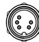
AISG 8-pin male interface with 5 loaded contacts
