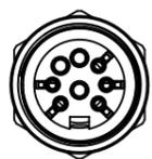
AISG 8-pin female interface with 5 loaded contacts
