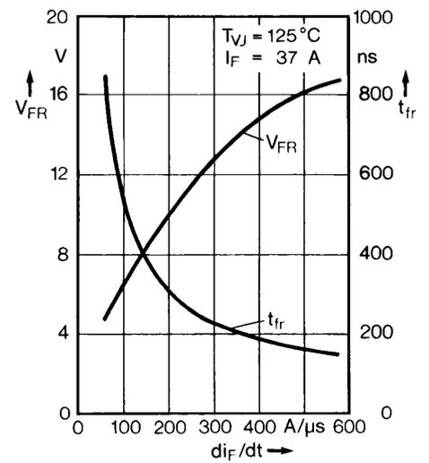
Fig. 6 Peak forward voltage versus  $di_F/dt$ .
