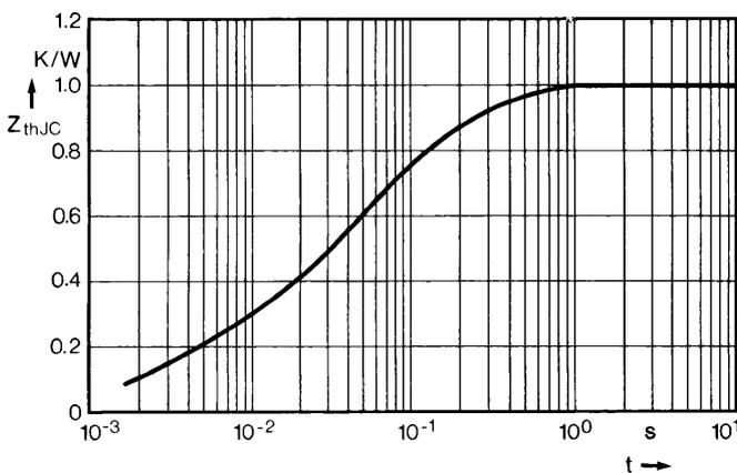
Fig. 7 Transient thermal impedance junction to case.
