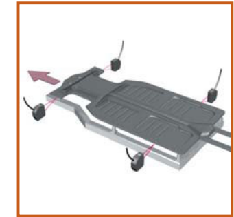
Measuring Car Body Widths (ZS-HLDS10)
