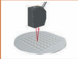
Measuring Electrode Thickness on Compound Semiconductors
