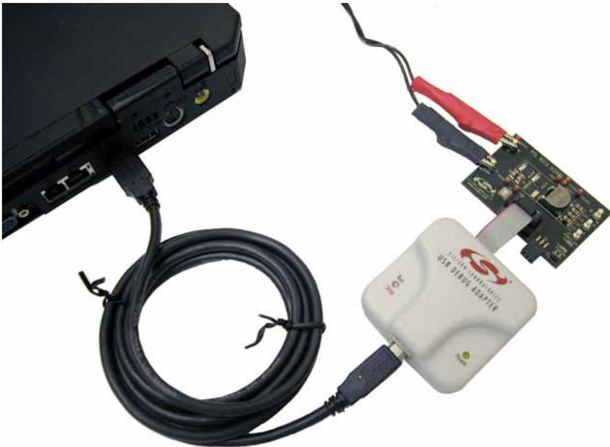
Figure 3. Overall View of the Debug Connection (Load not Connected)
