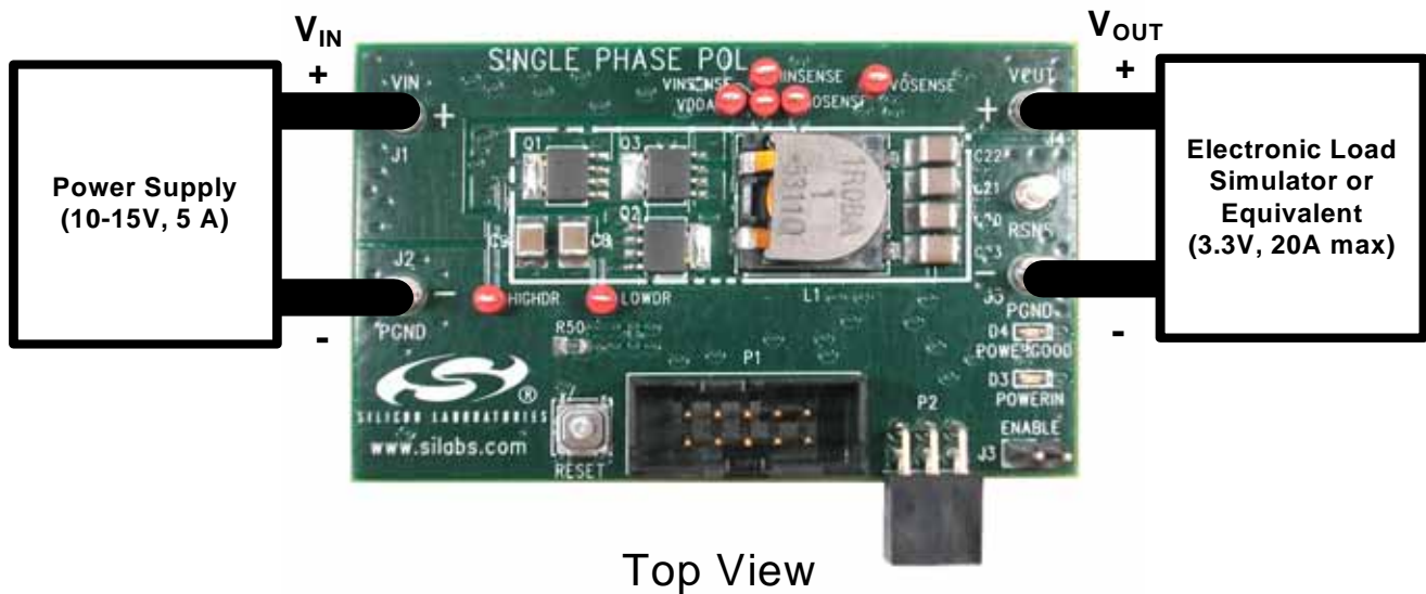
Figure 2. Board Power Configuration
