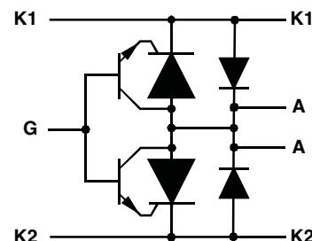
Terminals K1, K2 and A correspond to the alternative line designators of T, R and G or A, B and C. The negative protection voltage is controlled by the voltage,  $V_{GG}$ , applied to the G terminal.
