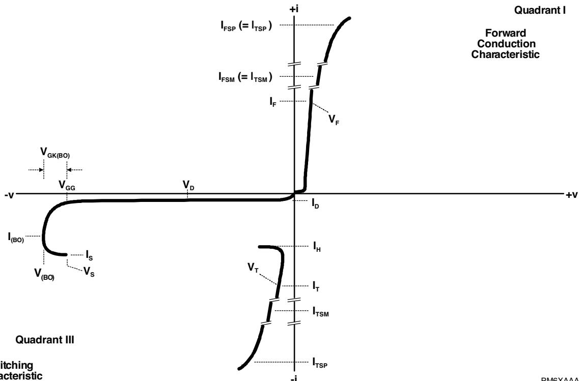
**Figure 1. Voltage-Current Characteristic**
