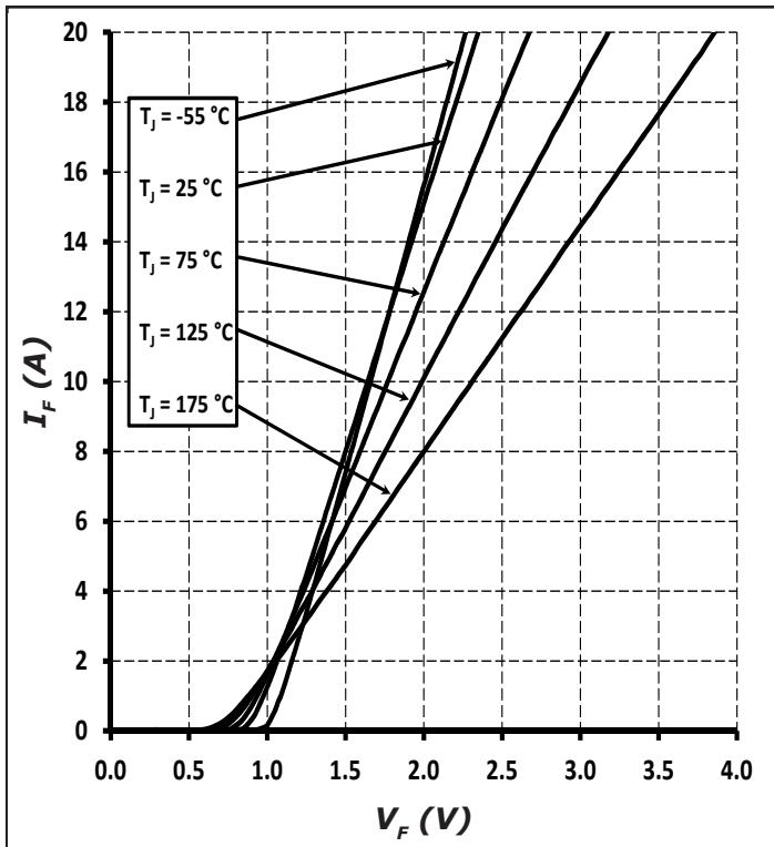
Figure 1. Forward Characteristics
