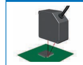
Inspecting for Board Coplanarity
