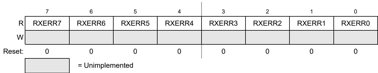
Figure 18-18. MSCAN Receive Error Counter (CANRXERR)
