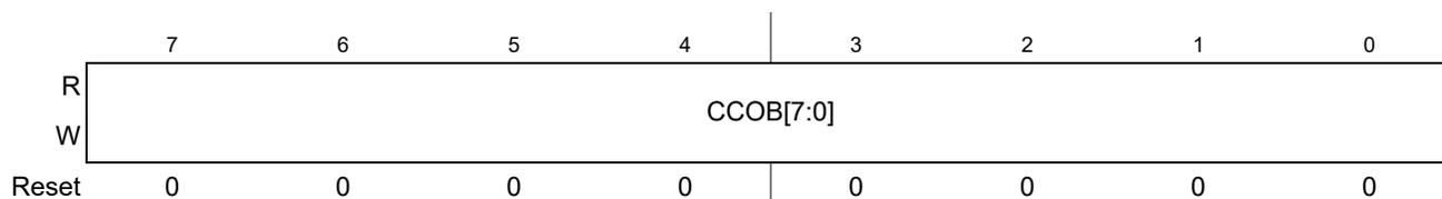
Figure 22-29. Flash Common Command Object 5 Low Register (FCCOB5LO)
