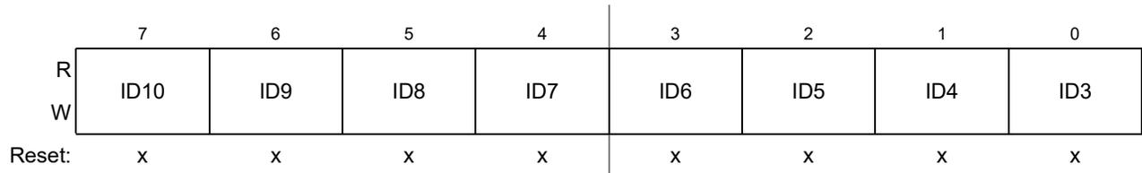
Figure 18-30. Identifier Register 0 — Standard Mapping
