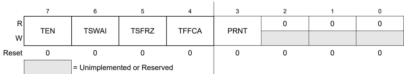
Figure 11-12. Timer System Control Register 1 (TSCR1)
