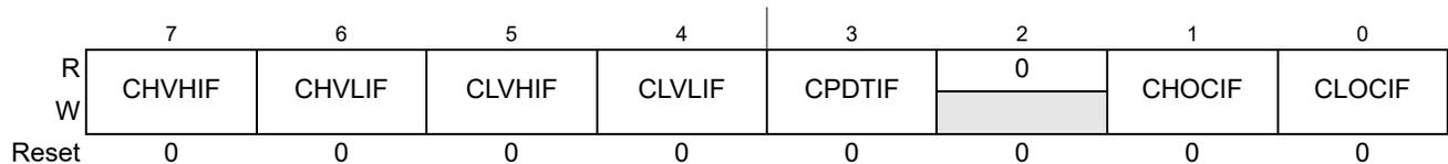
Figure 17-9. CAN Physical Layer Interrupt Flag Register (CPIF)
