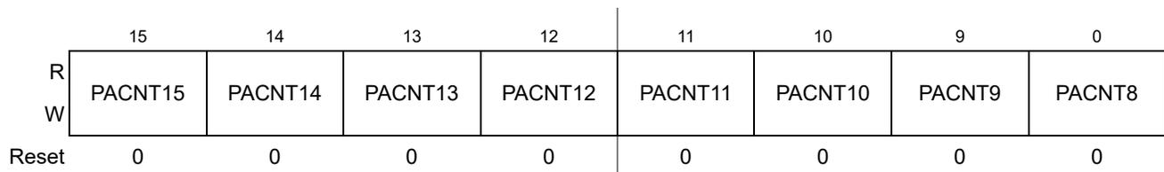
Figure 11-26. Pulse Accumulator Count Register High (PACNTH)
