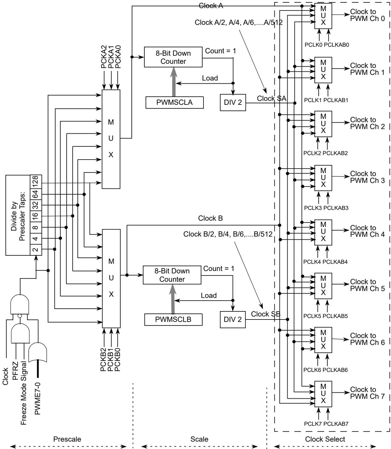
Figure 13-15. PWM Clock Select Block Diagram
