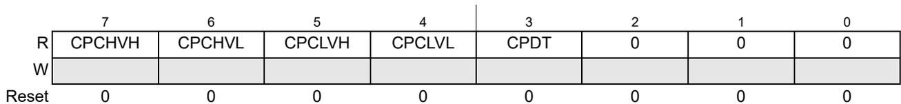
Figure 17-5. CAN Physical Layer Status Register (CPSR)
