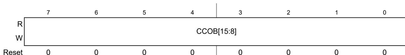
Figure 22-28. Flash Common Command Object 5 High Register (FCCOB5HI)
