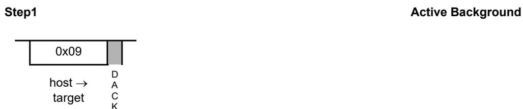
This command is used to step through application code. In active BDM this command executes the next CPU instruction in application code. If enabled an ACK is driven.
