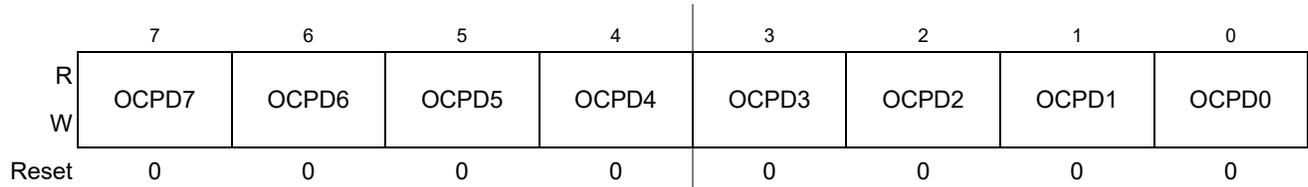
Figure 11-28. Output Compare Pin Disconnect Register (OCPD)
