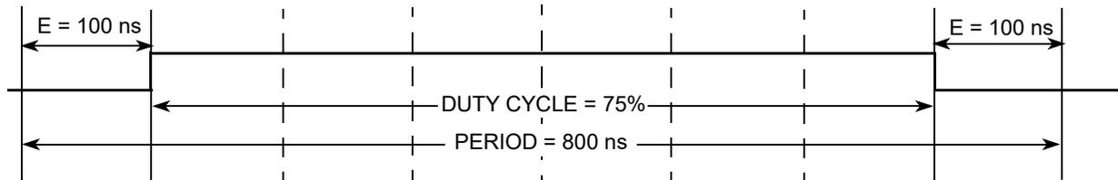
Figure 13-20. PWM Center Aligned Output Example Waveform
