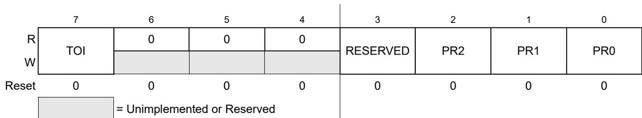
Figure 12-15. Timer System Control Register 2 (TSCR2)s12tim16b4c
