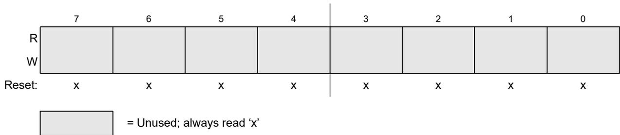
Figure 18-33. Identifier Register 3 — Standard Mapping
