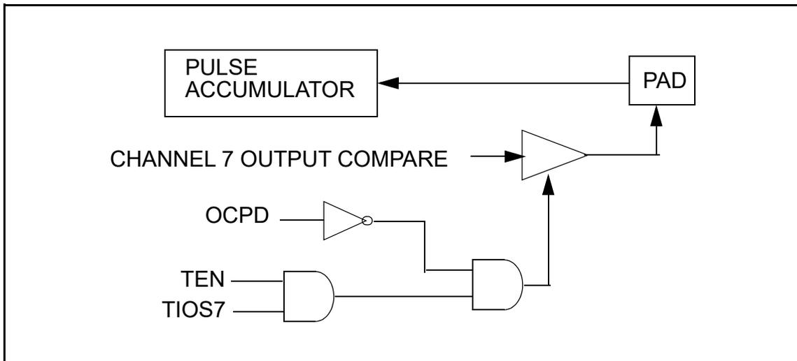
Figure 11-4. Channel 7 Output Compare/Pulse Accumulator Logic
