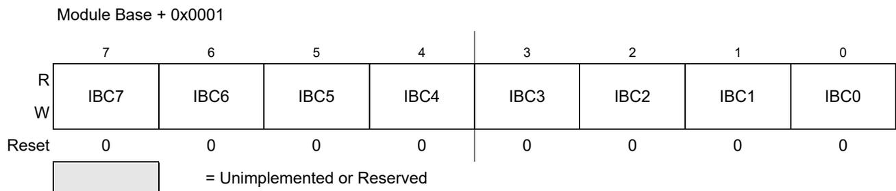
Figure 16-4. IIC Bus Frequency Divider Register (IBFD)
