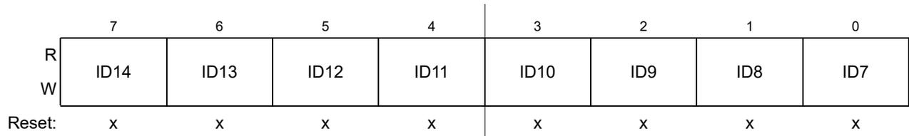
Figure 18-28. Identifier Register 2 (IDR2) — Extended Identifier Mapping
