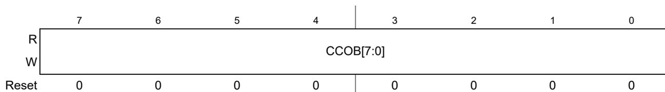
Figure 22-19. Flash Common Command Object 0 Low Register (FCCOB0LO)
