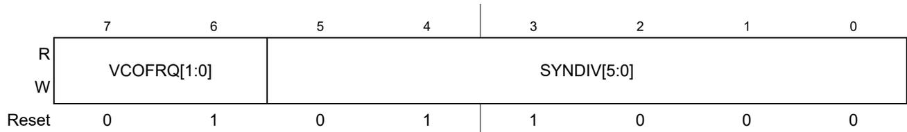
Figure 8-5. S12CPMU\_UHV\_V7 Synthesizer Register (CPMUSYNR)
