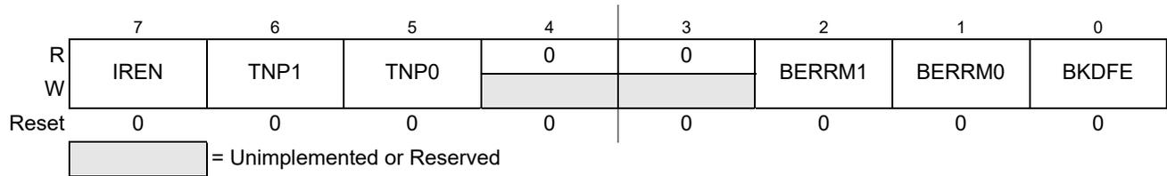
Figure 14-8. SCI Alternative Control Register 2 (SCIACR2)
