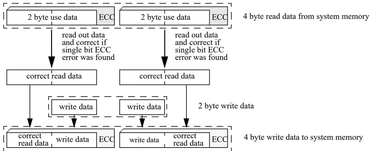
Figure 7-9. 2 byte non-aligned write access
