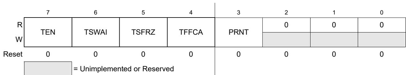
Figure 12-8. Timer System Control Register 1 (TSCR1)
