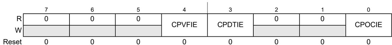
Figure 17-8. CAN Physical Layer Interrupt Enable Register (CPIE)
