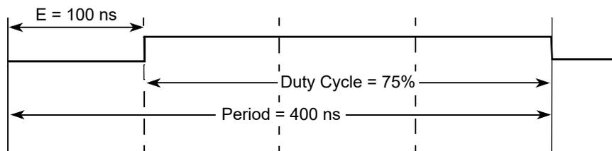
**Figure 13-18. PWM Left Aligned Output Example Waveform**
