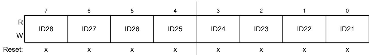
Figure 18-26. Identifier Register 0 (IDR0) — Extended Identifier Mapping
