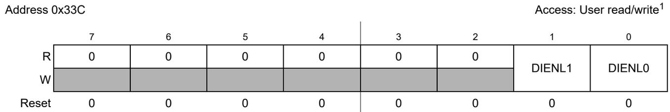
Figure 2-29. Port L Digital Input Enable Register (DIENL)
