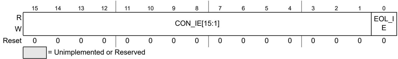
**Figure 9-14. ADC Conversion Interrupt Enable Register (ADCCONIE)**
