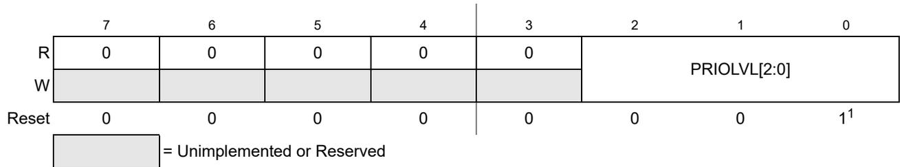
**Figure 5-7. Interrupt Request Configuration Data Register 2 (INT\_CFDATA2)**
