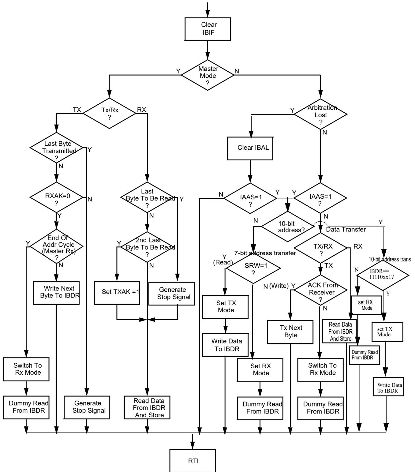
Figure 16-16. Flow-Chart of Typical IIC Interrupt Routine
