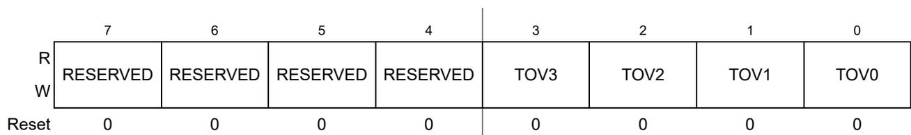
Figure 12-9. Timer Toggle On Overflow Register 1 (TTOV)
