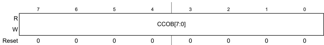
**Figure 22-23. Flash Common Command Object 2 Low Register (FCCOB2LO)**
