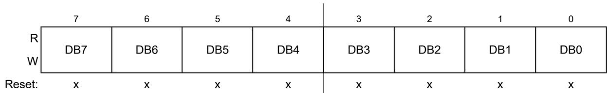
Figure 18-34. Data Segment Registers (DSR0–DSR7) — Extended Identifier Mapping
