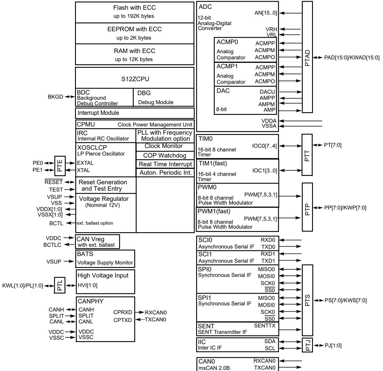
Block Diagram shows the maximum configuration!
