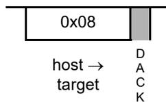
This command is used to exit active BDM and begin (or resume) execution of CPU application code. The CPU pipeline is flushed and refilled before normal instruction execution resumes. Prefetching begins at the current address in the PC. If any register (such as the PC) is altered by a BDC command whilst in BDM, the updated value is used when prefetching resumes. If enabled, an ACK is driven on exiting active BDM.
