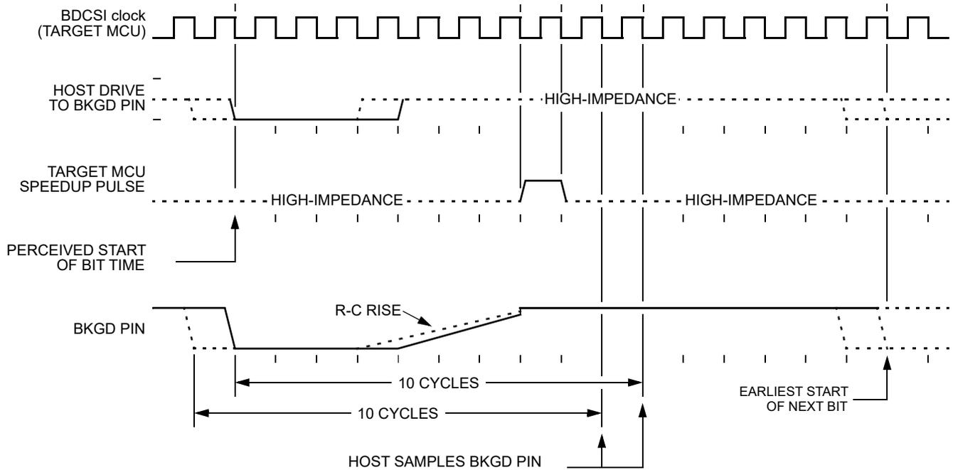
**Figure 3-7. BDC Target-to-Host Serial Bit Timing (Logic 1)**
