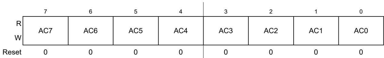
**Figure 18-20. MSCAN Identifier Acceptance Registers (First Bank) — CANIDAR0–CANIDAR3**
