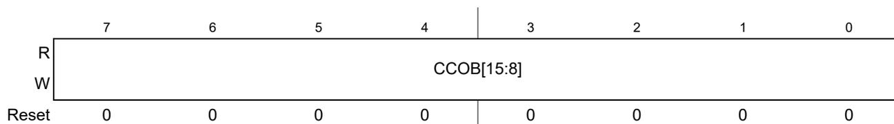
Figure 22-22. Flash Common Command Object 2 High Register (FCCOB2HI)
