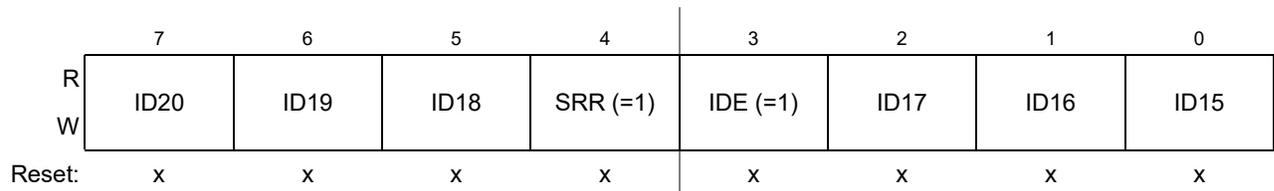
Figure 18-27. Identifier Register 1 (IDR1) — Extended Identifier Mapping
