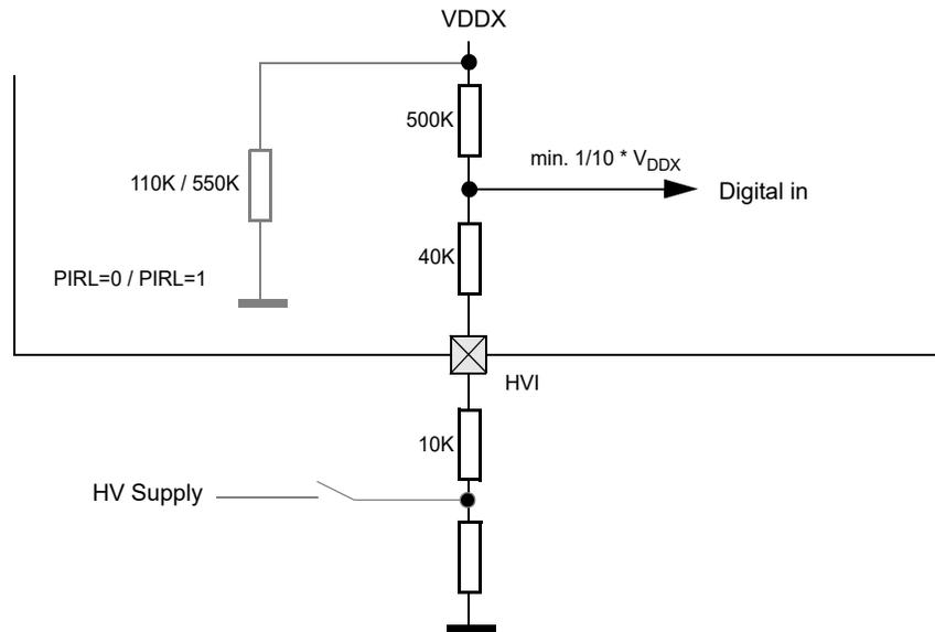
**Figure 2-36. Digital Input Read with Pullup Enabled**
