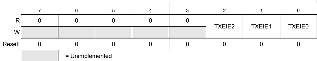
Figure 18-11. MSCAN Transmitter Interrupt Enable Register (CANTIER)
