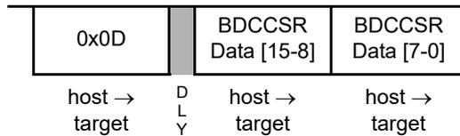
16-bit write to the BDCCSR register. No ACK pulse is generated. Writing to this register can be used to configure control bits or clear flag bits. Refer to the register bit descriptions.
