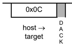
This command is used to exit active BDM and begin (or resume) execution of application code. The CPU pipeline is flushed and refilled before normal instruction execution resumes. Prefetching begins at the current address in the PC. If any register (such as the PC) is altered by a BDC command whilst in BDM, the updated value is used when prefetching resumes.
