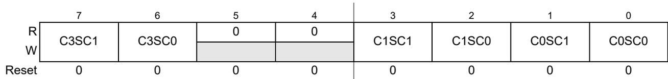
Figure 6-8. Debug State Control Register 3 (DBGSCR3)
