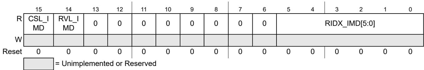
**Figure 9-16. ADC Intermediate Result Information Register (ADCIMDRI)**
