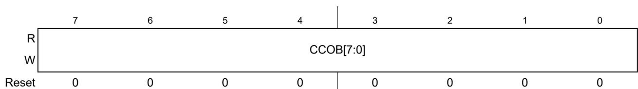
**Figure 22-27. Flash Common Command Object 4 Low Register (FCCOB4LO)**
