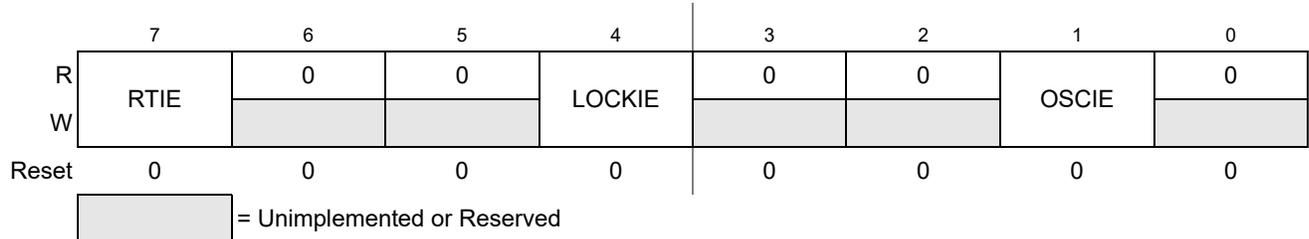
**Figure 8-9. S12CPMU\_UHV\_V7 Interrupt Enable Register (CPMUINT)**
