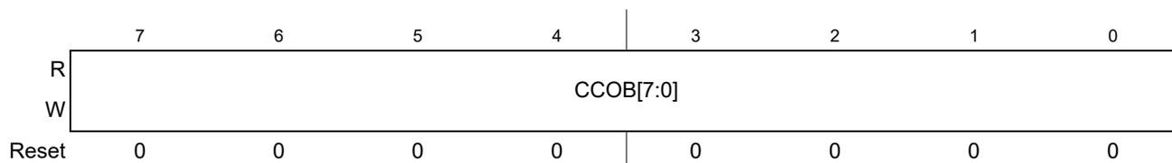
Figure 22-21. Flash Common Command Object 1 Low Register (FCCOB1LO)
