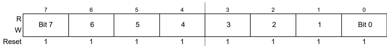
**Figure 13-14. PWM Channel Duty Registers (PWMDTY<sub>x</sub>)**
