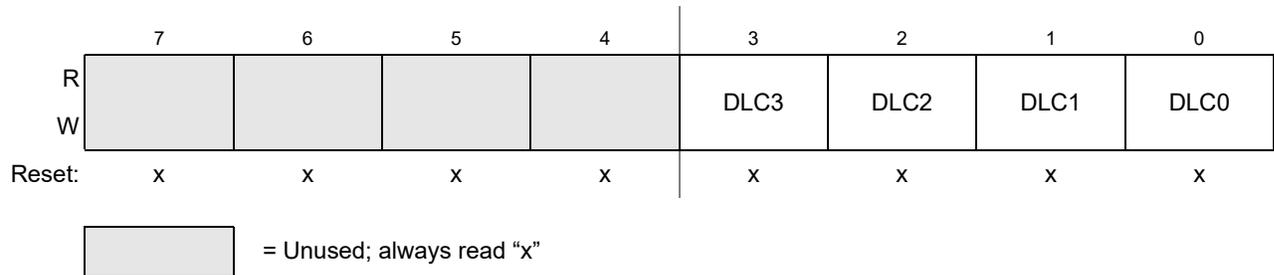
**Figure 18-35. Data Length Register (DLR) — Extended Identifier Mapping**
