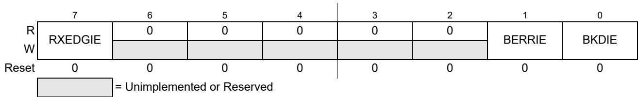
Figure 14-7. SCI Alternative Control Register 1 (SCIACR1)
