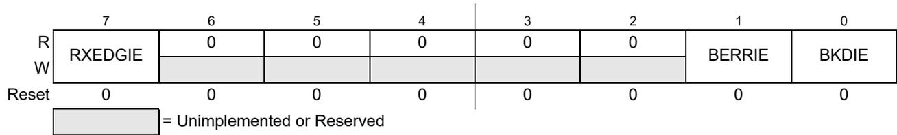
**Figure 14-7. SCI Alternative Control Register 1 (SCIACR1)**
