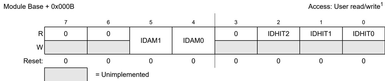
**Figure 18-15. MSCAN Identifier Acceptance Control Register (CANIDAC)**
