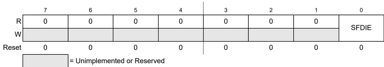
Figure 22-10. Flash Error Configuration Register (FERCNFG)
