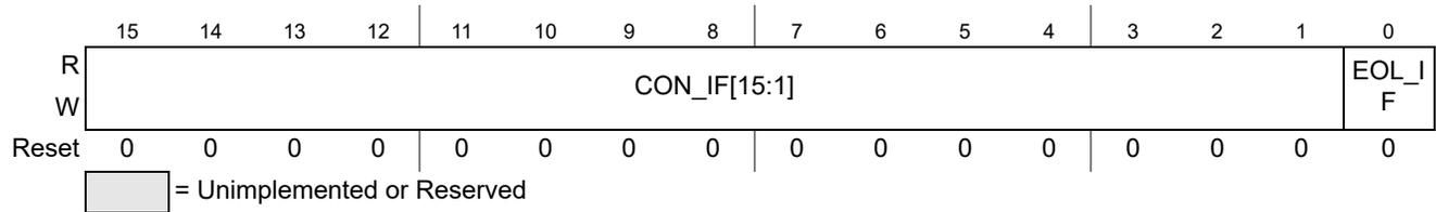
Figure 9-15. ADC Conversion Interrupt Flag Register (ADCCONIF)
