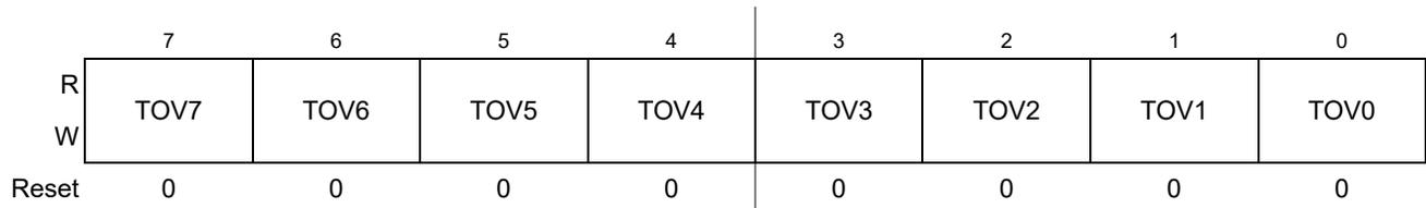
Figure 11-13. Timer Toggle On Overflow Register 1 (TTOV)
