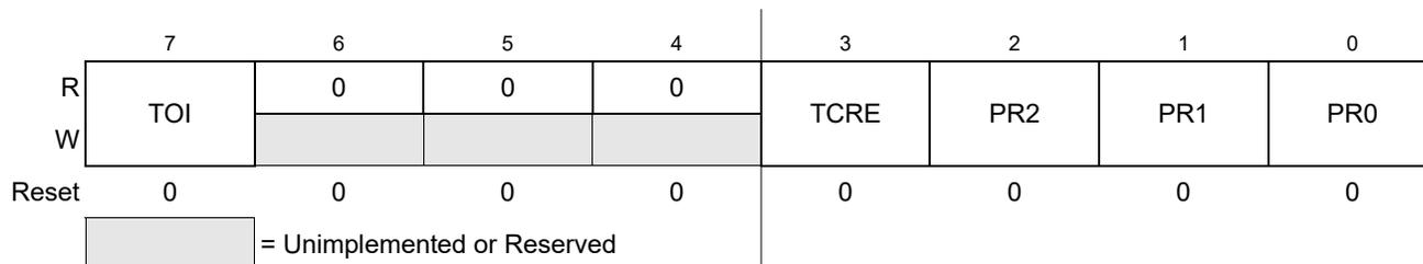
Figure 11-19. Timer System Control Register 2 (TSCR2)
