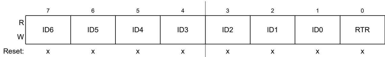
Figure 18-29. Identifier Register 3 (IDR3) — Extended Identifier Mapping
