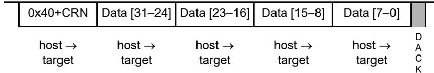
If the device is in active BDM, this command writes the 32-bit operand to the selected CPU general-purpose register. See [Section 3.4.5.1, “BDC Access Of CPU Registers](#) for the CRN details. Accesses to CPU registers are always 32-bits wide, regardless of implemented register width. If enabled an ACK pulse is generated after the internal write access has been completed or aborted.
