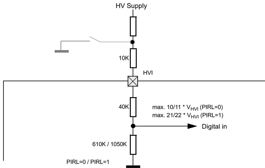
Figure 2-37. Digital Input Read with Pulldown Enabled
