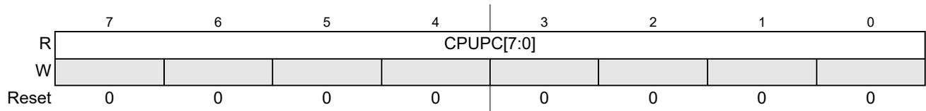
**Figure 4-7. Captured S12ZCPU Program Counter (MMCPCH, MMPCM, MMCPCL)**
