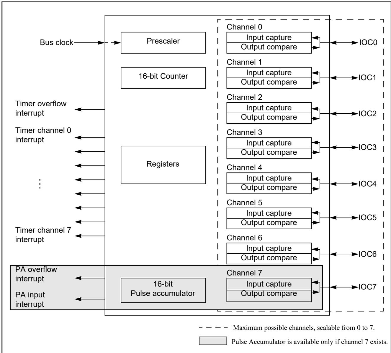
Figure 11-1. TIM16B8CV3 Block Diagram
