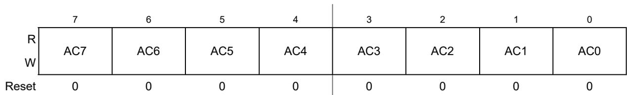
**Figure 18-21. MSCAN Identifier Acceptance Registers (Second Bank) — CANIDAR4–CANIDAR7**
