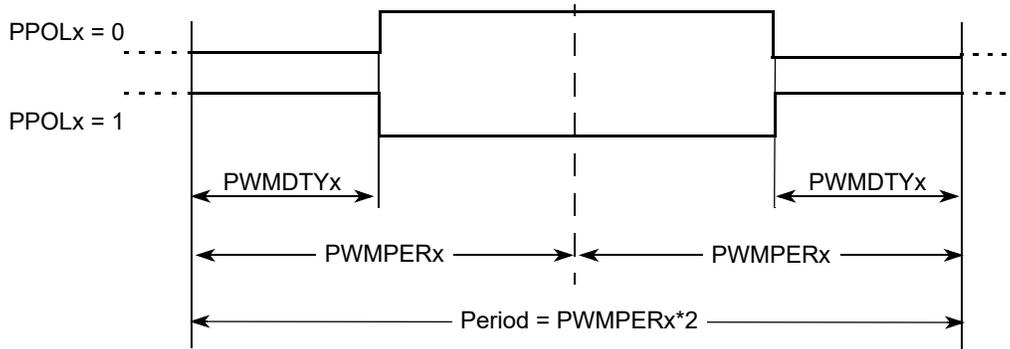
Figure 13-19. PWM Center Aligned Output Waveform
