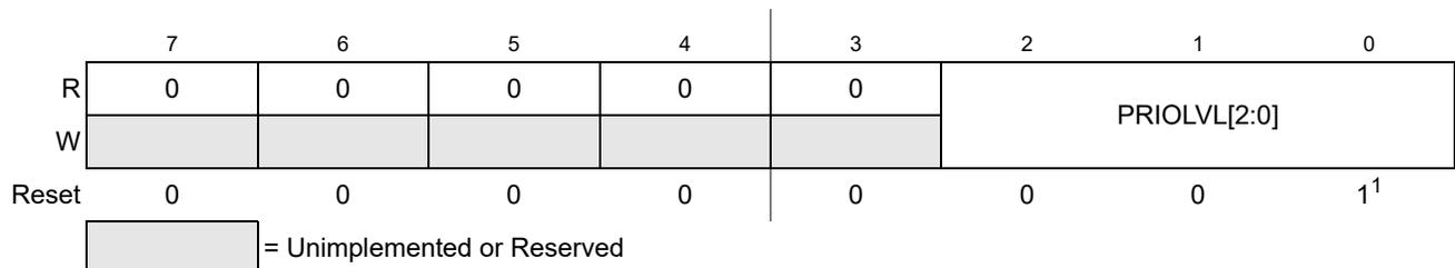
Figure 5-5. Interrupt Request Configuration Data Register 0 (INT\_CFDATA0)
