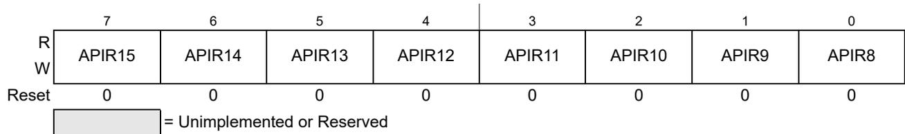
**Figure 8-23. Autonomous Periodical Interrupt Rate High Register (CPMUAPIRH)**
