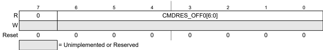
**Figure 9-26. ADC Command and Result Offset Register 0 (ADCCROFF0)**
