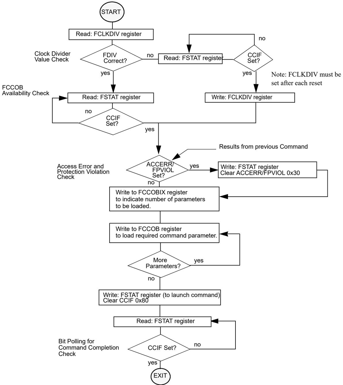
Figure 22-30. Generic Flash Command Write Sequence Flowchart
