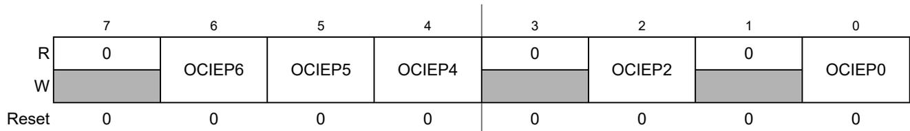
Figure 2-22. Port P Over-Current Interrupt Enable Register
