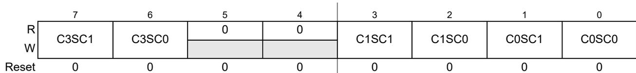
Figure 6-6. Debug State Control Register 1 (DBGSCR1)
