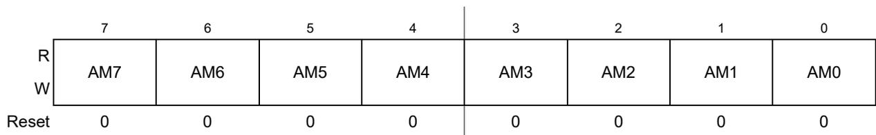
**Figure 18-22. MSCAN Identifier Mask Registers (First Bank) — CANIDMR0–CANIDMR3**<sup>1</sup> Read: Anytime
