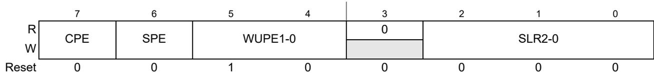
Figure 17-3. CAN Physical Layer Control Register (CPCR)
