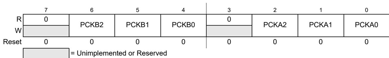
**Figure 13-6. PWM Prescale Clock Select Register (PWMPRCLK)**
