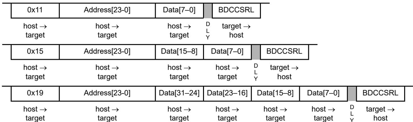
Write data to the specified memory address. The address is transmitted as three 8-bit packets (msb to lsb) immediately after the command.
