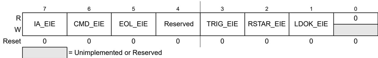
**Figure 9-10. ADC Error Interrupt Enable Register (ADCEIE)**
