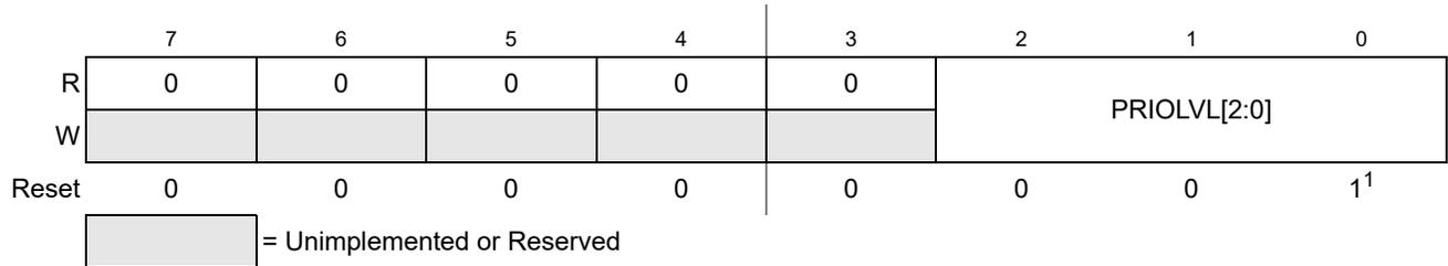
**Figure 5-8. Interrupt Request Configuration Data Register 3 (INT\_CFDATA3)**
