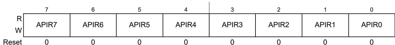
**Figure 8-24. Autonomous Periodical Interrupt Rate Low Register (CPMUAPIRL)**
