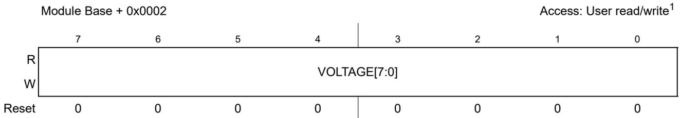
Figure 19-4. Analog Output Voltage Level Register (DACVOL)
