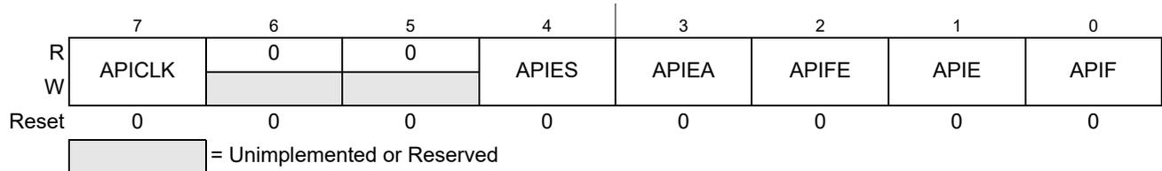
**Figure 8-20. Autonomous Periodical Interrupt Control Register (CPMUAPICTL)**
