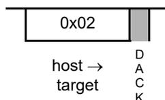
Enables the hardware handshake protocol in the serial communication. The hardware handshake is implemented by an acknowledge (ACK) pulse issued by the target MCU in response to a host command.
