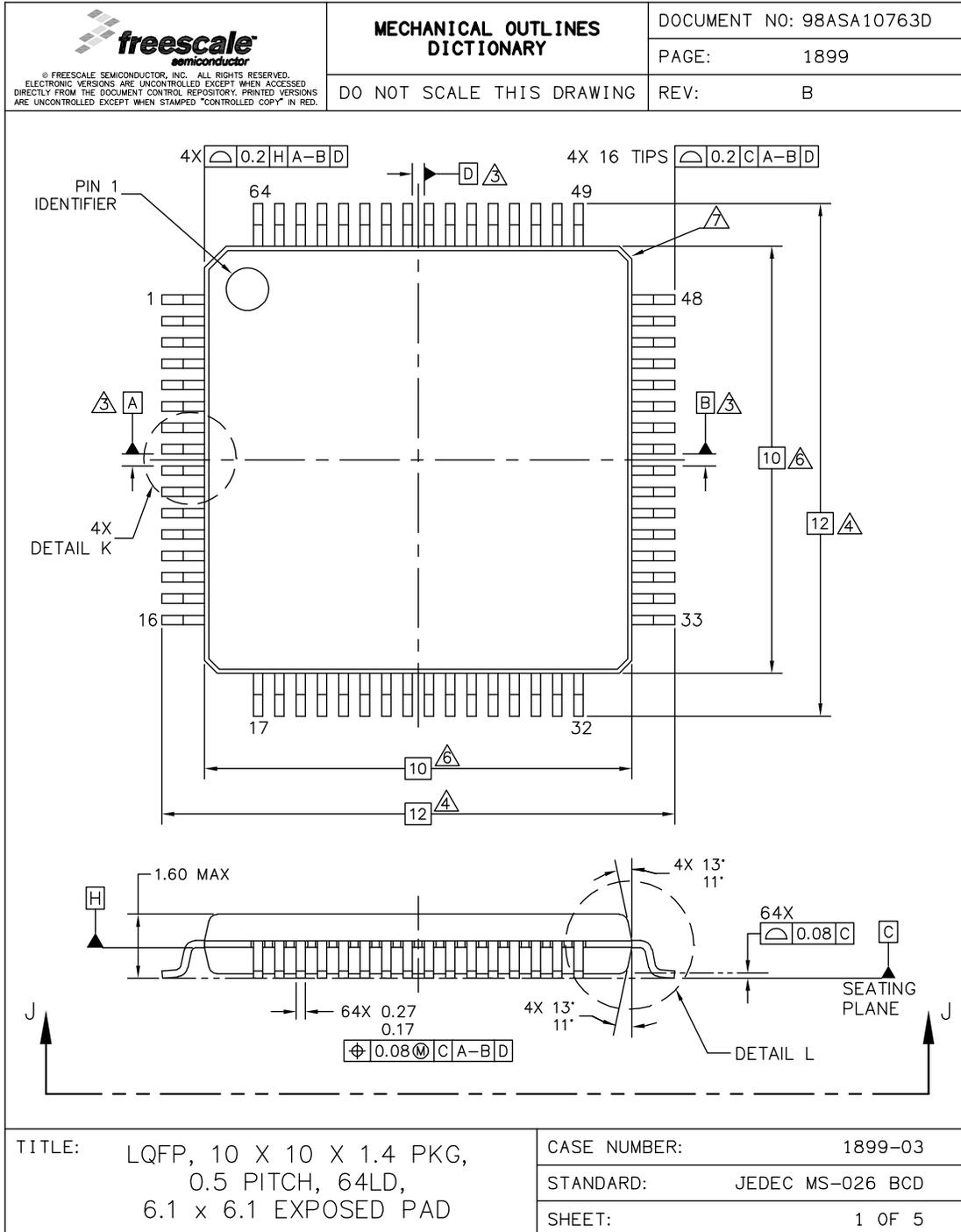
Figure L-2. 64 LQFP Exposed Pad Package
