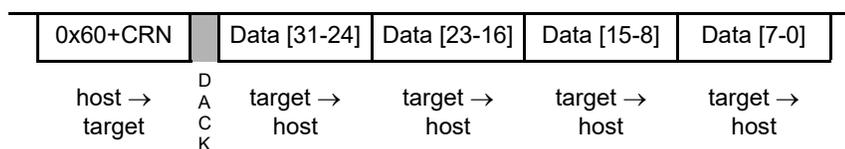
This command reads the selected CPU registers and returns the 32-bit result. Accesses to CPU registers are always 32-bits wide, regardless of implemented register width. Bytes that are not implemented return zero. The register is addressed through the CPU register number (CRN). See [Section 3.4.5.1, “BDC](#)
