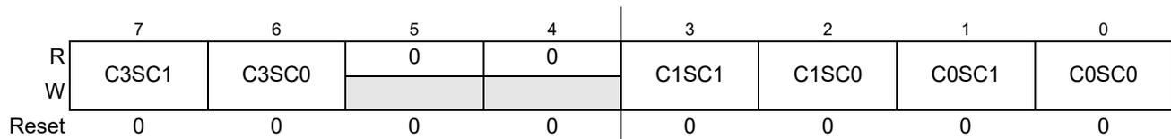
**Figure 6-7. Debug State Control Register 2 (DBGSCR2)**
