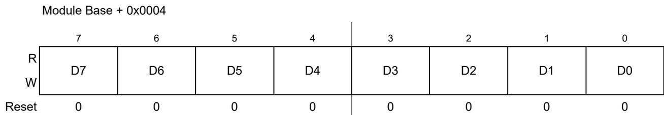
Figure 16-8. IIC Bus Data I/O Register (IBDR)
