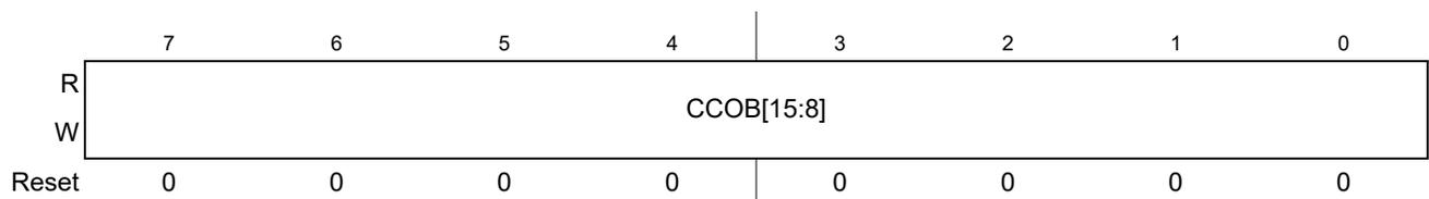
**Figure 22-26. Flash Common Command Object 4 High Register (FCCOB4HI)**
