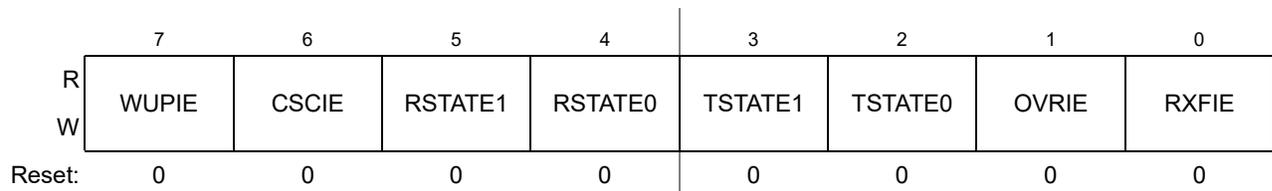
Figure 18-9. MSCAN Receiver Interrupt Enable Register (CANRIER)
