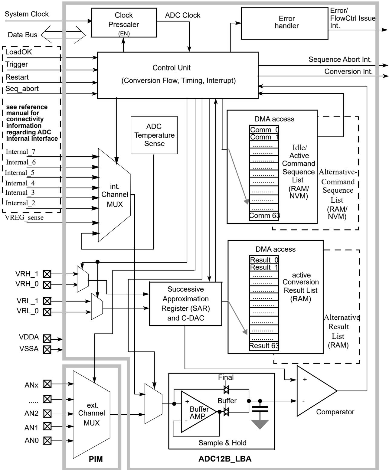
Figure 9-2. ADC12B\_LBA Block Diagram
