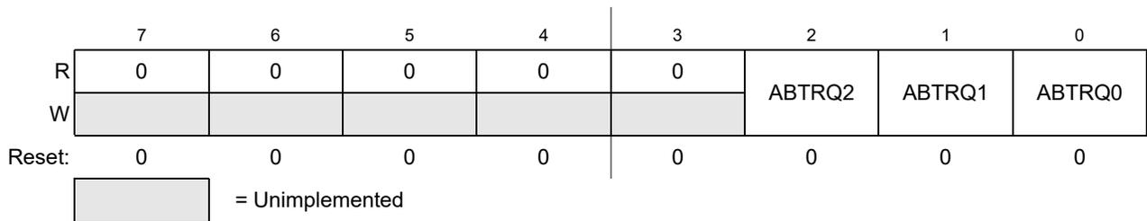
**Figure 18-12. MSCAN Transmitter Message Abort Request Register (CANTARQ)**
