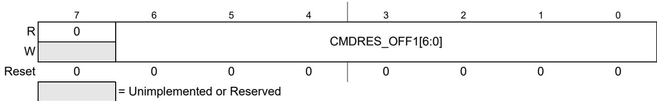
**Figure 9-27. ADC Command and Result Offset Register 1 (ADCCROFF1)**
