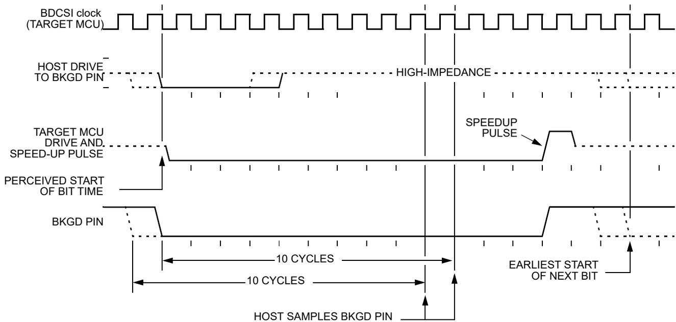
Figure 3-8. BDC Target-to-Host Serial Bit Timing (Logic 0)
