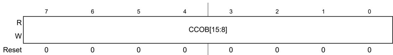
**Figure 22-24. Flash Common Command Object 3 High Register (FCCOB3HI)**
