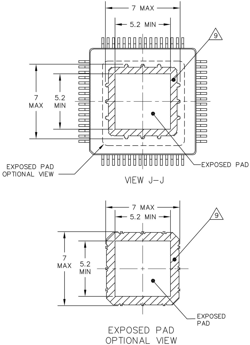
Figure L-3. 64 LQFP Exposed Pad Package
