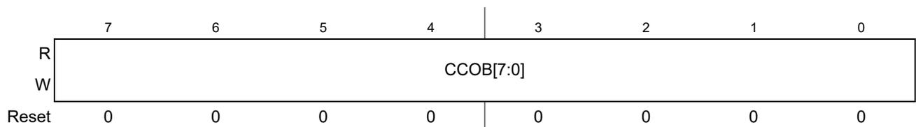
**Figure 22-25. Flash Common Command Object 3 Low Register (FCCOB3LO)**
