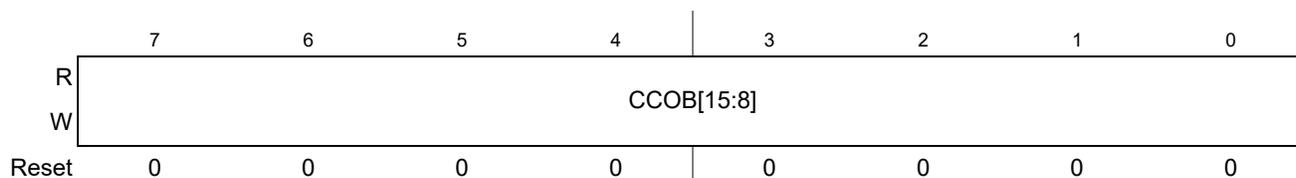
Figure 22-18. Flash Common Command Object 0 High Register (FCCOB0HI)
