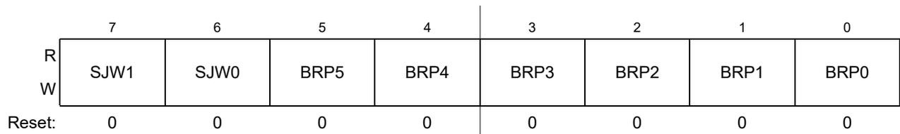
**Figure 18-6. MSCAN Bus Timing Register 0 (CANBTR0)**
