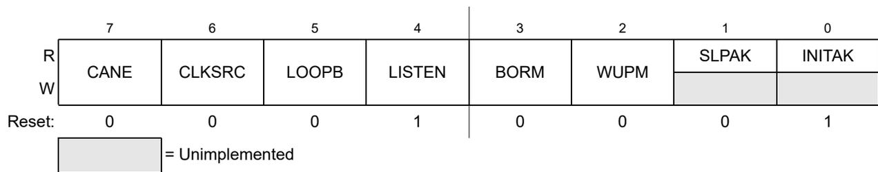
**Figure 18-5. MSCAN Control Register 1 (CANCTL1)**<sup>1</sup> Read: Anytime
