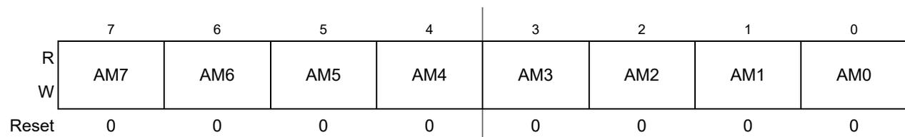
**Figure 18-23. MSCAN Identifier Mask Registers (Second Bank) — CANIDMR4–CANIDMR7**
