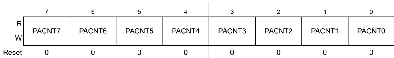
Figure 11-27. Pulse Accumulator Count Register Low (PACNTL)
