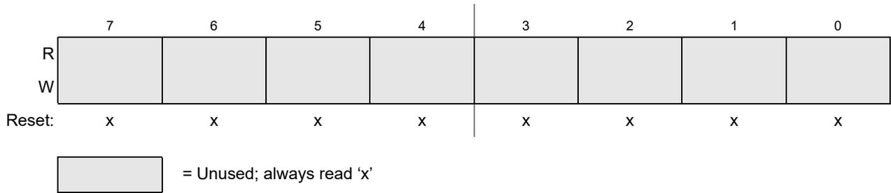
Figure 18-32. Identifier Register 2 — Standard Mapping
