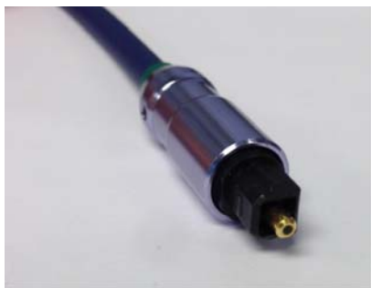
Figure 34. TOSLINK Connector and Optical Fiber Cable for the S/PDIF Input and Output
