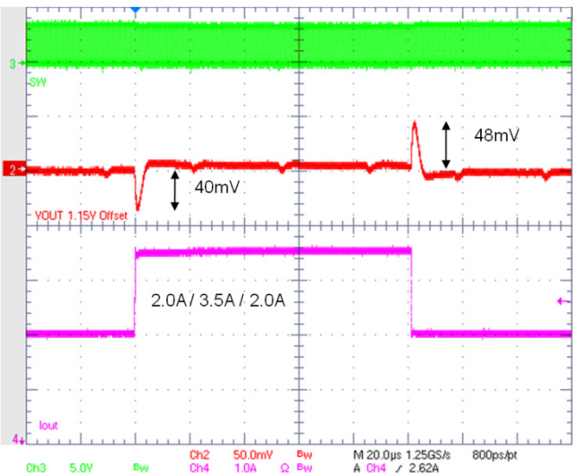
Figure 32. Transient Load 2.0 – 3.5 A Auto Mode
