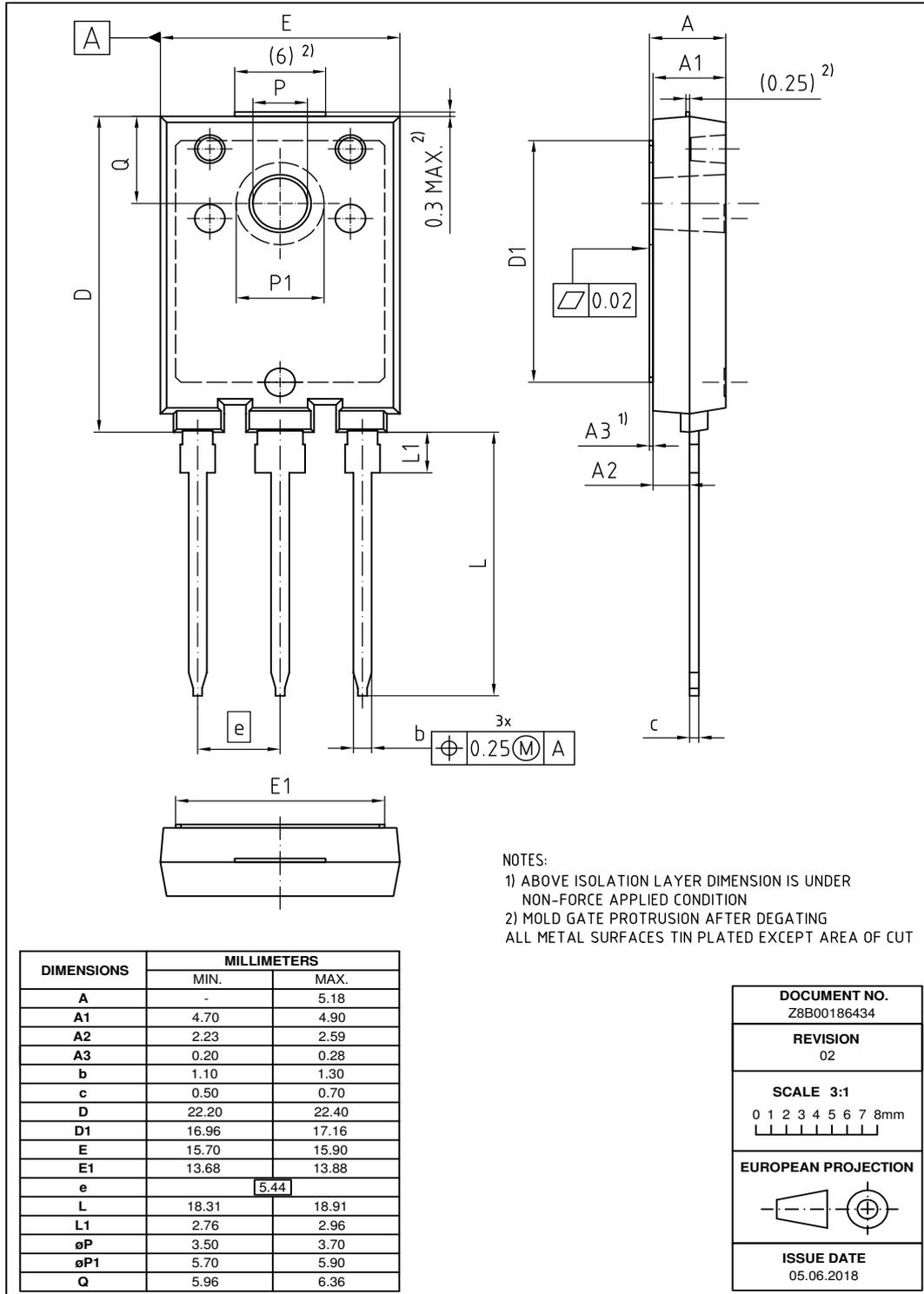
Note: For a proper handling and assembly of the advanced isolation device in the application the isolation layer must not be exposed to potential penetration via sharp implements or mechanical impacts/shocks, which exceed levels indicated in International Standard (IEC60068-2-6 and IEC60068-2-27). The advanced isolation device is intended only to be used assembled on an appropriate heatsink with recommended flatness of <20µm per 100mm and roughness of <10µm.
