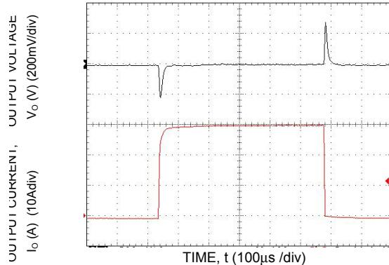
**Figure 22. Transient Response to Dynamic Load Change from 0% to 50% with  $V_{IN}=12V$ .**
