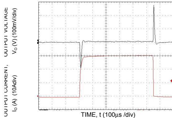
**Figure 10. Transient Response to Dynamic Load Change from 0% to 50% with  $V_{IN}=12V$ .**
