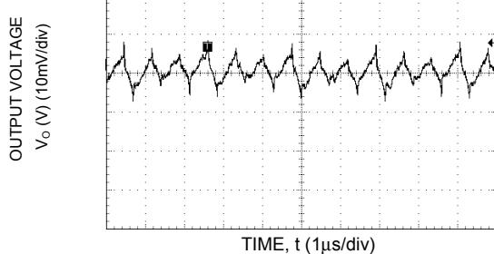
**Figure 21. Typical output ripple and noise ( $V_{IN} = 12V$ ,  $I_o = I_{o,max}$ ).**
