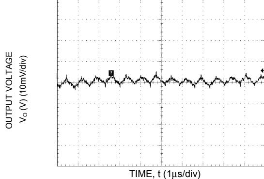
**Figure 3. Typical output ripple and noise ( $V_{IN} = 12V$ ,  $I_{o,max}$ ).**
