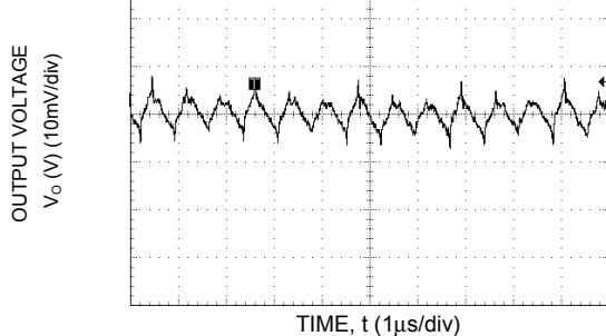
**Figure 9. Typical output ripple and noise ( $V_{IN} = 12V$ ,  $I_o = I_{o,max}$ ).**
