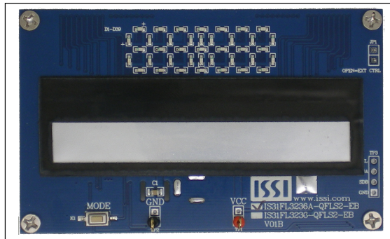
Figure 1: Photo of IS31FL3236/IS31FL3236A Evaluation Board
