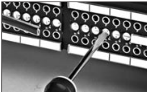
Center Strip Removes For Normaling Access
