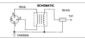
Series 9000 Line Matching Transformers offer low-loss interconnections between high and low impedance equipment. Exclusive mu-metal shielding protects against spurious electrostatic and RF fields. Units are bi-directional and can be used as follows:
