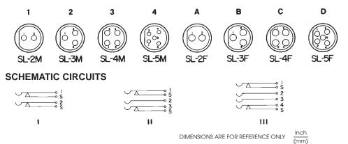
Receptacle Housings: Die-cast zinc, nickel-plated. Cord Plug Housings: Copper alloy, nickel-plated.
