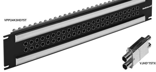
The VPP Series video patchbays offer a wide variety of options for video patching. The HD Series meets SMPTE 292M specifications for high definition video signaling, covering a bandwidth range from DC to 2.4GHz. The SD Series is perfect for serial digital, with a bandwidth from DC to 1.75GHZ. Both come in either terminated or non-terminated, 24 or 26 jacks, 1.75" or 3.5" heights.
