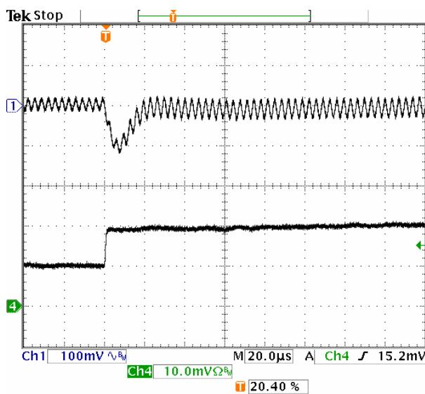
**Fig-2.5V-6:** Output voltage response for  $V_{out}=2.5V$  to positive load current step-change from 5A to 10A with slew rate of  $5A/\mu s$  at  $V_{in}=5.0V$ .  $C_o=47\mu Fx2$  ceramic.
