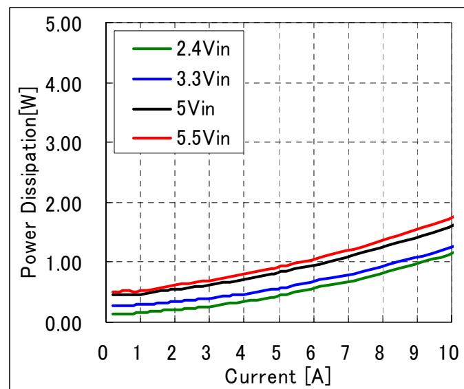
**Fig-1.5V-3:** Power dissipation vs. load current and input voltage for  $V_{out}=1.5V$ .
