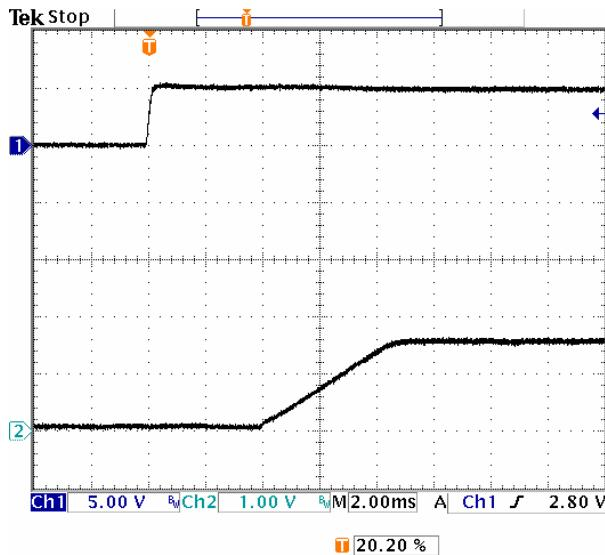
**Fig-1.5V-4:** Turn-on transient for  $V_{out}=1.5V$  with application of  $V_{in}$  at full rated load current (resistive) and  $47\mu Fx2$  external capacitance at  $V_{in}=5.0V$ .
