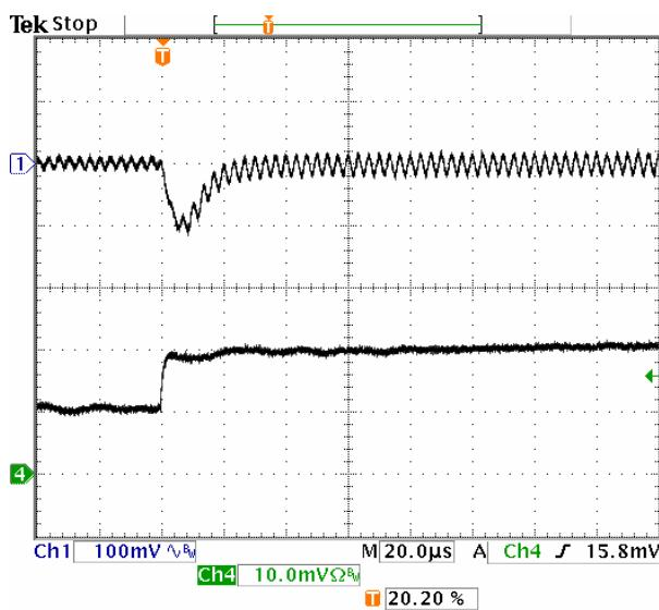
**Fig-1.0V-6:** Output voltage response for  $V_{out}=1.0V$  to positive load current step-change from 5A to 10A with slew rate of  $5A/\mu s$  at  $V_{in}=5.0V$ .  $C_o=47\mu Fx2$  ceramic.
