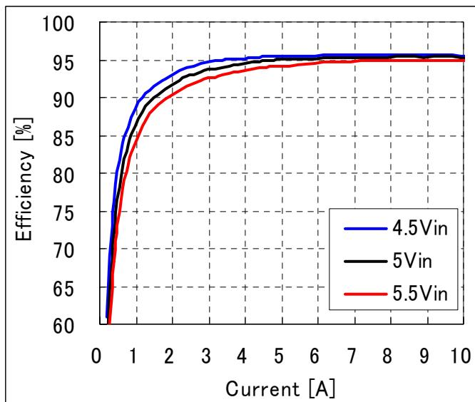
**Fig-3.3V-2:** Efficiency vs. load current and input voltage for  $V_{out}=3.3V$ .
