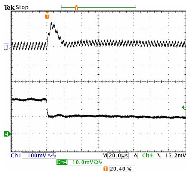
**Fig-3.3V-7:** Output voltage response for  $V_{out}=3.3V$  to negative load current step-change from 10A to 5A with slew rate of  $-5A/\mu s$  at  $V_{in}=5.0V$ .  $C_o=47\mu Fx2$  ceramic.
