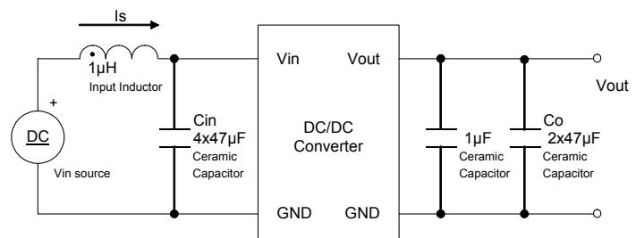
Fig. H: Test setup for measuring input reflected ripple current
