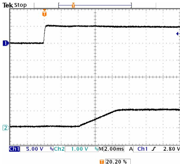
**Fig-1.0V-4:** Turn-on transient for  $V_{out}=1.0V$  with application of  $V_{in}$  at full rated load current (resistive) and  $47\mu Fx2$  external capacitance at  $V_{in}=5.0V$ .
