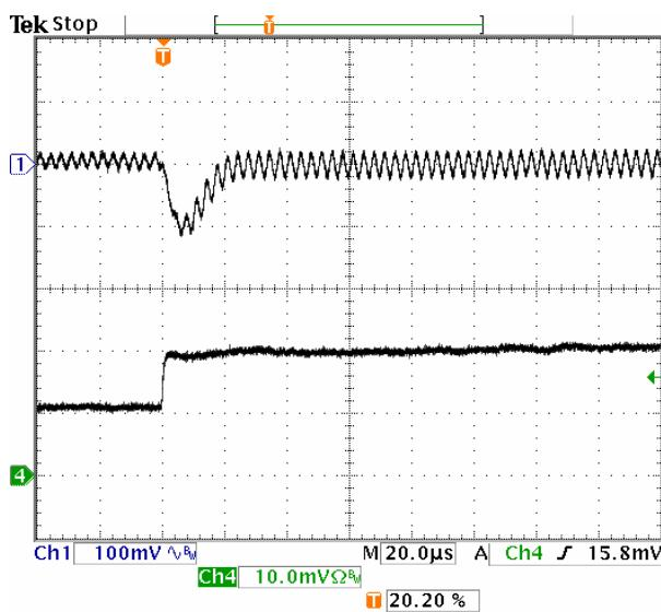
**Fig-1.5V-6:** Output voltage response for  $V_{out}=1.5V$  to positive load current step-change from 5A to 10A with slew rate of  $5A/\mu s$  at  $V_{in}=5.0V$ .  $C_o=47\mu Fx2$  ceramic.
