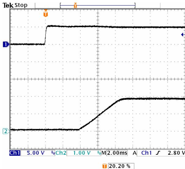
**Fig-1.8V-4:** Turn-on transient for  $V_{out}=1.8V$  with application of  $V_{in}$  at full rated load current (resistive) and  $47\mu Fx2$  external capacitance at  $V_{in}=5.0V$ .
