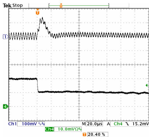
**Fig-2.5V-7:** Output voltage response for  $V_{out}=2.5V$  to positive load current step-change from 10A to 5A with slew rate of  $-5A/\mu s$  at  $V_{in}=5.0V$ .  $C_o=47\mu Fx2$  ceramic.
