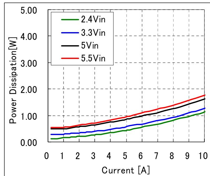
**Fig-1.8V-3:** Power dissipation vs. load current and input voltage for  $V_{out}=1.8V$ .
