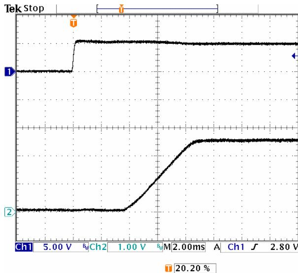
**Fig-2.5V-4:** Turn-on transient for  $V_{out}=2.5V$  with application of  $V_{in}$  at full rated load current (resistive) and  $47\mu Fx2$  external capacitance at  $V_{in}=5.0V$ .
