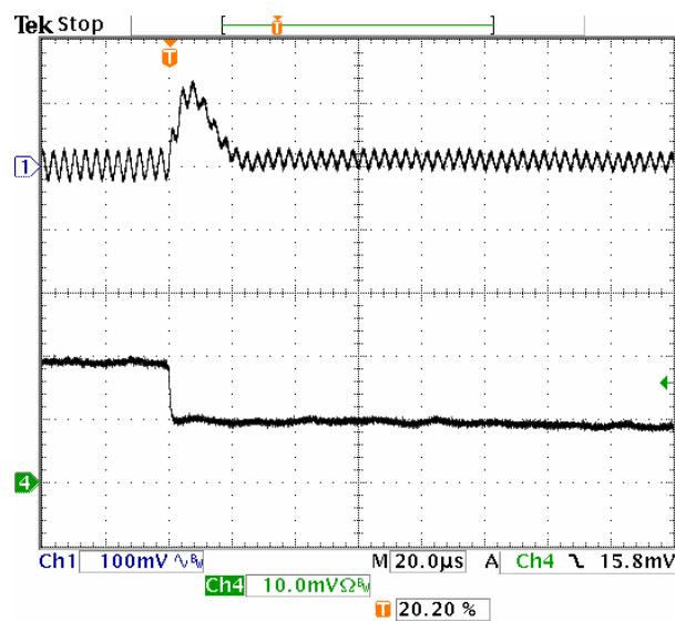
**Fig-2.0V-7:** Output voltage response for  $V_{out}=2.0V$  to positive load current step-change from 10A to 5A with slew rate of  $-5A/\mu s$  at  $V_{in}=5.0V$ .  $C_o=47\mu Fx2$  ceramic.
