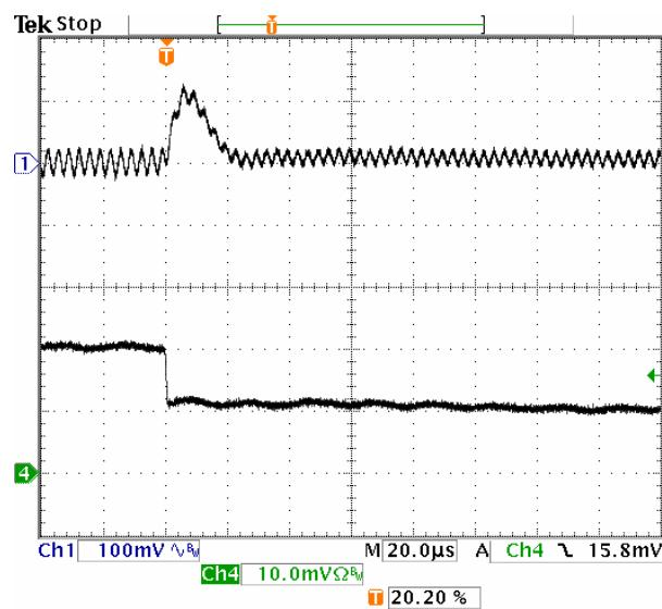
**Fig-1.5V-7:** Output voltage response for  $V_{out}=1.5V$  to positive load current step-change from 10A to 5A with slew rate of  $-5A/\mu s$  at  $V_{in}=5.0V$ .  $C_o=47\mu Fx2$  ceramic.
