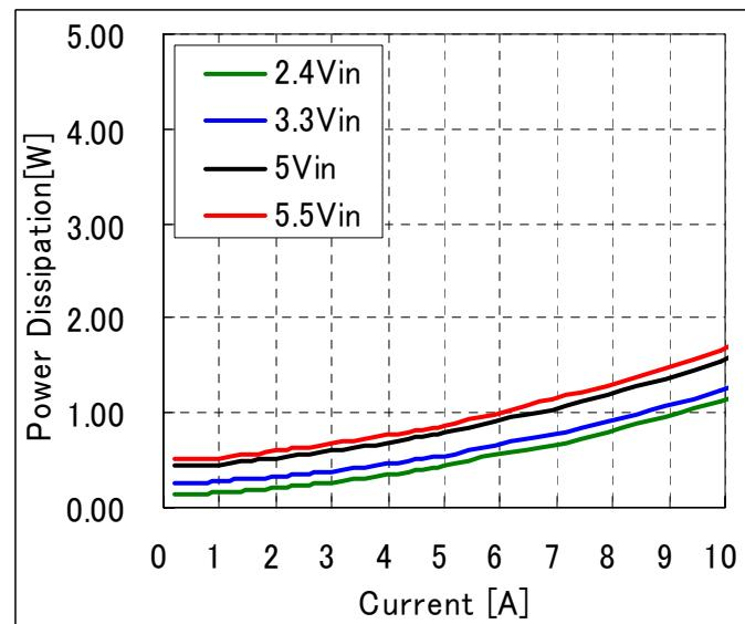
**Fig-1.0V-3:** Power dissipation vs. load current and input voltage for  $V_{out}=1.0V$ .
