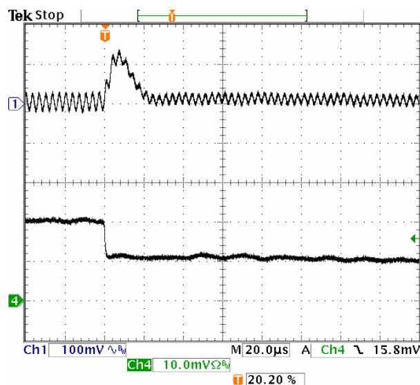
**Fig-1.8V-7:** Output voltage response for  $V_{out}=1.8V$  to positive load current step-change from 10A to 5A with slew rate of  $-5A/\mu s$  at  $V_{in}=5.0V$ .  $C_o=47\mu Fx2$  ceramic.
