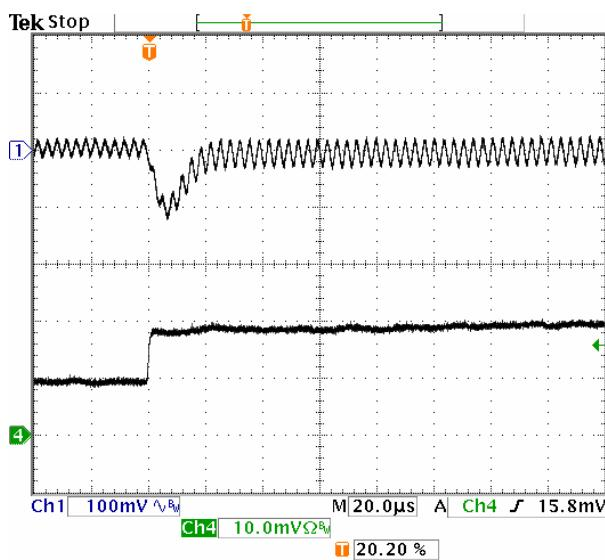
**Fig-2.0V-6:** Output voltage response for  $V_{out}=2.0V$  to positive load current step-change from 5A to 10A with slew rate of  $5A/\mu s$  at  $V_{in}=5.0V$ .  $C_o=47\mu Fx2$  ceramic.
