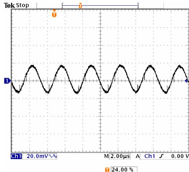
**Fig-1.0V-5:** Output voltage ripple (20mV/div.) for  $V_{out}=1.0V$  at full rated load current into a resistive load with external capacitance  $47\mu Fx2$  ceramic +  $1\mu F$  ceramic at  $V_{in}=5.0V$ .
