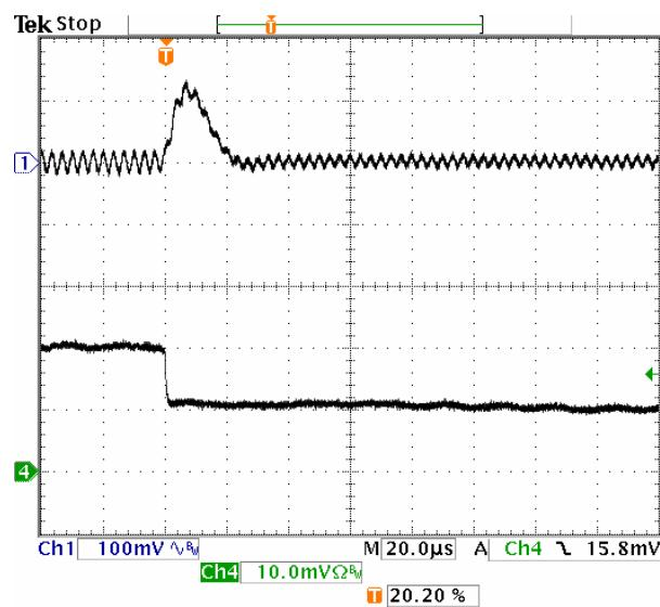
**Fig-1.0V-7:** Output voltage response for  $V_{out}=1.0V$  to positive load current step-change from 10A to 5A with slew rate of  $-5A/\mu s$  at  $V_{in}=5.0V$ .  $C_o=47\mu Fx2$  ceramic.
