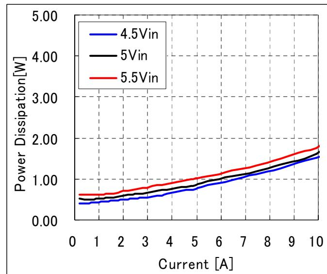
**Fig-3.3V-3:** Power dissipation vs. load current and input voltage for  $V_{out}=3.3V$ .
