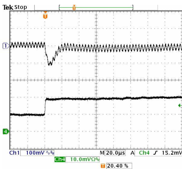
**Fig-3.3V-6:** Output voltage response for  $V_{out}=3.3V$  to positive load current step-change from 5A to 10A with slew rate of  $5A/\mu s$  at  $V_{in}=5.0V$ .  $C_o=47\mu Fx2$  ceramic.
