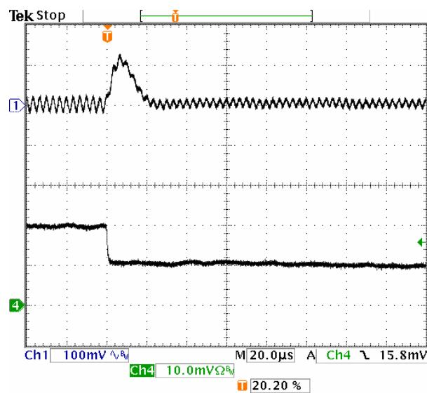
**Fig-1.2V-7:** Output voltage response for  $V_{out}=1.2V$  to positive load current step-change from 10A to 5A with slew rate of  $-5A/\mu s$  at  $V_{in}=5.0V$ .  $C_o=47\mu Fx2$  ceramic.
