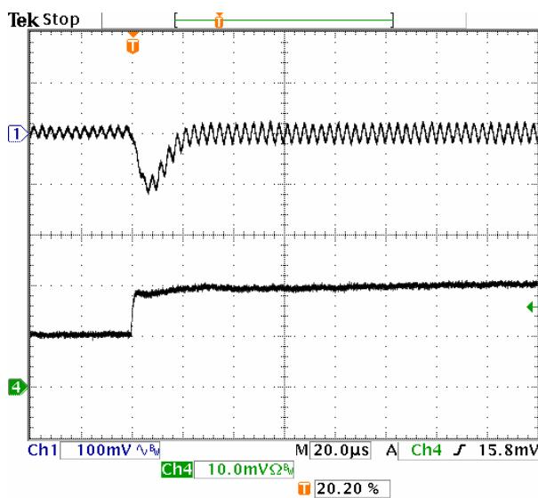
**Fig-1.2V-6:** Output voltage response for  $V_{out}=1.2V$  to positive load current step-change from 5A to 10A with slew rate of  $5A/\mu s$  at  $V_{in}=5.0V$ .  $C_o=47\mu Fx2$  ceramic.
