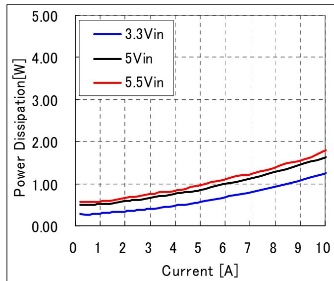
**Fig-2.0V-3:** Power dissipation vs. load current and input voltage for  $V_{out}=2.0V$ .
