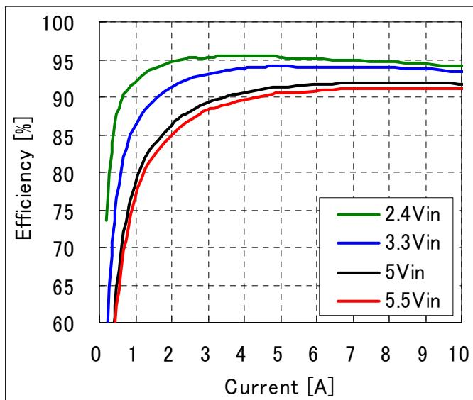
**Fig-1.8V-2:** Efficiency vs. load current and input voltage for  $V_{out}=1.8V$ .
