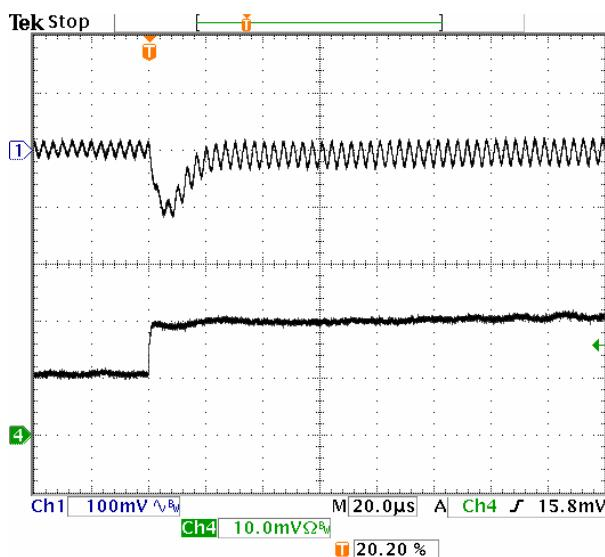
**Fig-1.8V-6:** Output voltage response for  $V_{out}=1.8V$  to positive load current step-change from 5A to 10A with slew rate of  $5A/\mu s$  at  $V_{in}=5.0V$ .  $C_o=47\mu Fx2$  ceramic.
