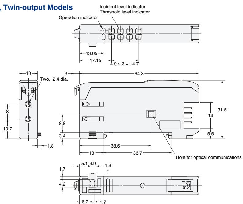
**Dimensions with Master Connector Connected**
