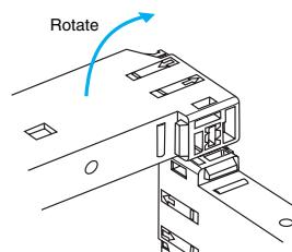
When using the E3X-DA-N with the Mobile Console, mount the End Plate in the way shown below.
