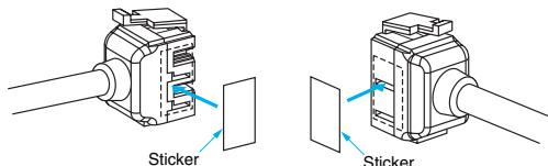
Note: Attach the stickers to the sides with grooves.
