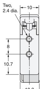
**With Mounting Bracket Attached**
