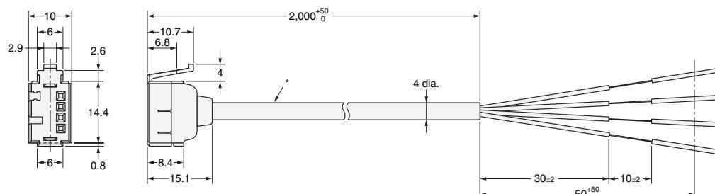
\* E3X-CN11: 4-dia. vinyl-insulated round cable with 3 conductors (Conductor cross section: 0.2 mm<sup>2</sup>; Insulation diameter: 1.1 mm).
