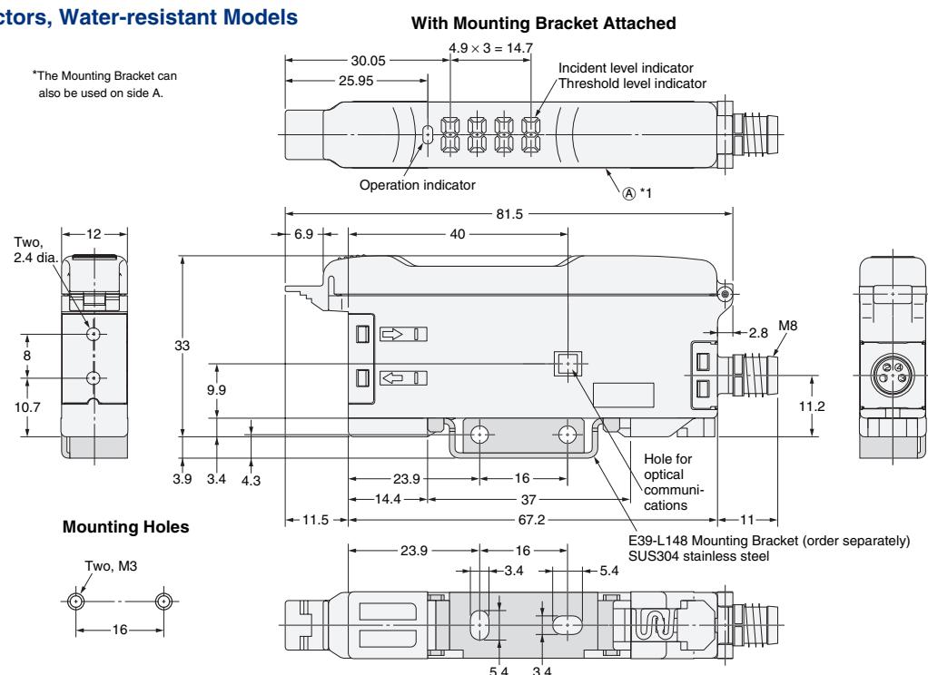
**Amplifiers with Standard Connectors, Twin-output Models**
