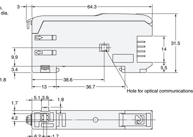
**Dimensions with Master Connector Connected**
