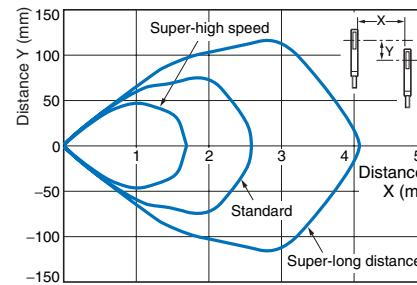
**Operating Range** With standard sensing object at maximum sensitivity. (Use for the positioning of the object and Sensor.)
