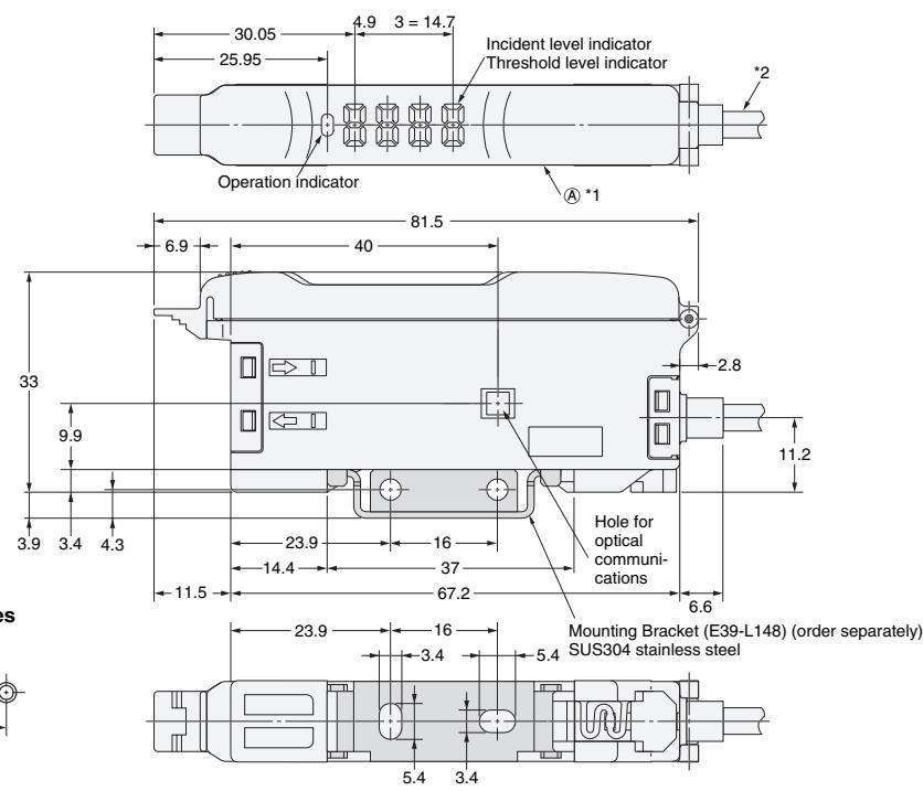
\*1. The Mounting Bracket can also be used on side A.
