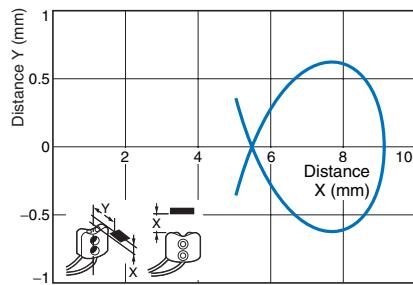
**Excess Gain Ratio vs. Distance** With standard sensing object at maximum sensitivity.
