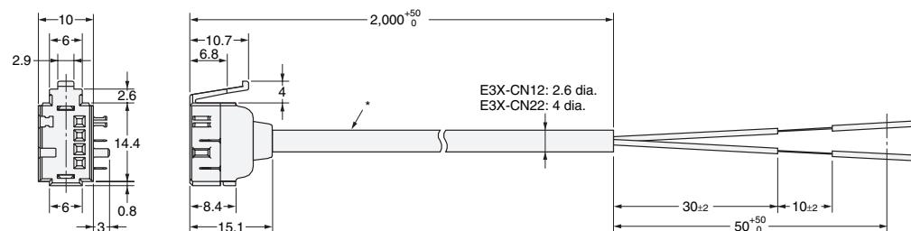
\* E3X-CN12: 2.6-dia. vinyl-insulated round cable with 1 conductor (Conductor cross section: 0.2 mm<sup>2</sup>; Insulation diameter: 1.1 mm).
