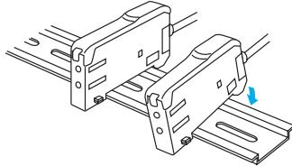
(2) Slide the Amplifiers together, line up the clips, and press the Amplifiers together until they click into place.
