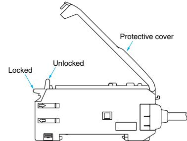
**Note: To maintain the fiber properties, confirm that the lock is released before removing the fiber.**
