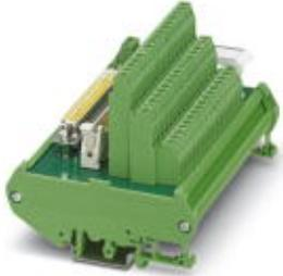
16-channel module for Honeywell C300 modules. The module is controlled by the control system via 37-pos. D-SUB or 50-pos. FLK. A screw connection is available in the field. Module width: 113 mm
