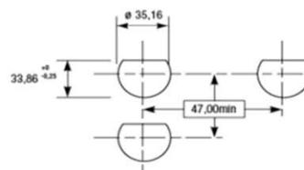
Jam nut receptacle rear panel mounting
