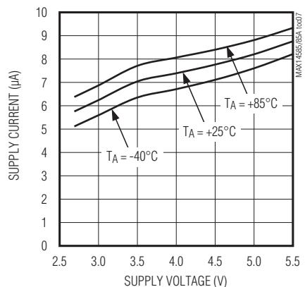
**V<sub>B</sub> SUPPLY CURRENT vs. SUPPLY VOLTAGE**
