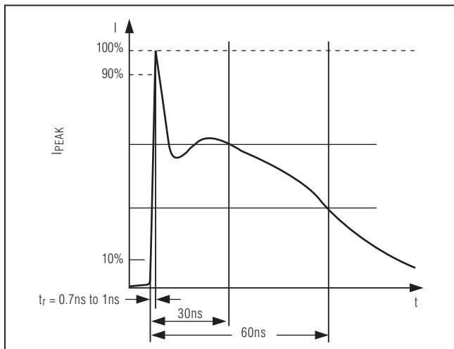
Figure 7. IEC 61000-4-2 ESD Generator Current Waveform
