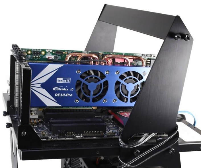
Figure 8-4 FPGA board installation on PC
