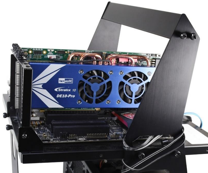
Figure 7-9 FPGA board installation on PC
