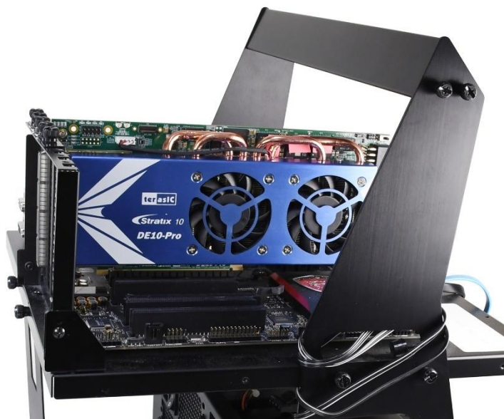
Figure 7-9 FPGA board installation on PC
