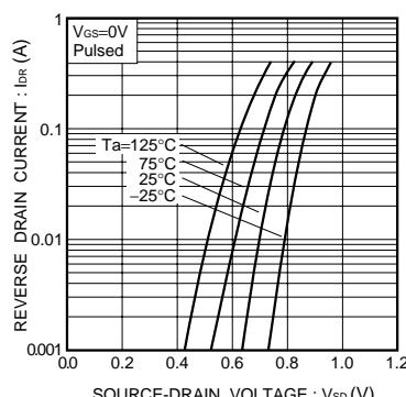
Fig.8 Reverse drain current vs. source-drain voltage ( I )
