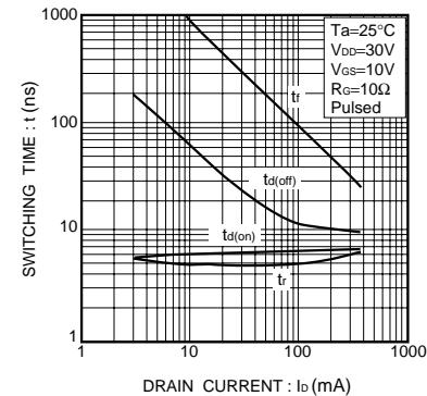
Fig.12 Switching characteristics
