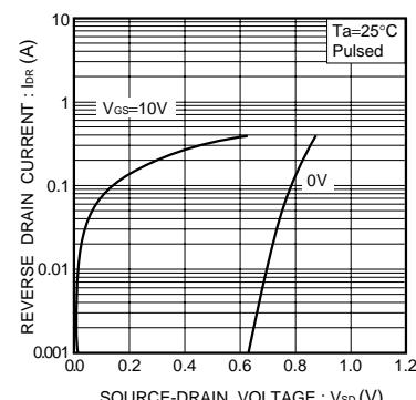
Fig.9 Reverse drain current vs. source-drain voltage ( II )
