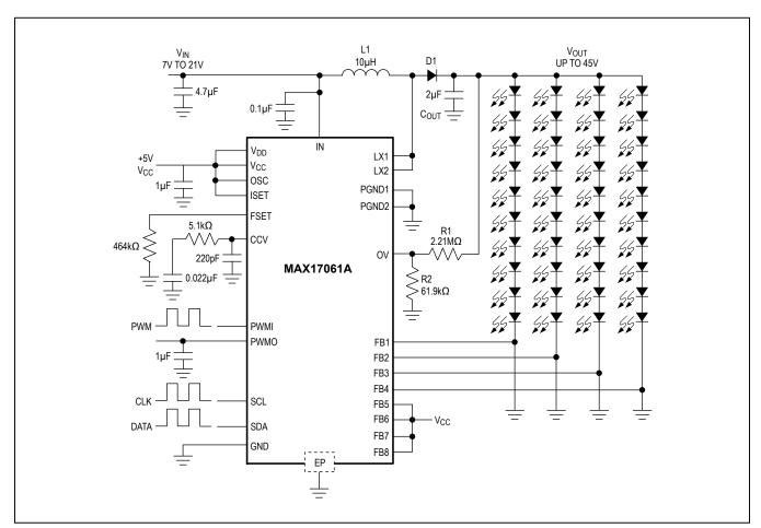
Figure 1. Typical Operating Circuit
