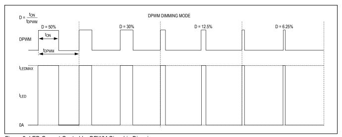
Figure 3. LED Current Control by DPWM Signal in Dimming
