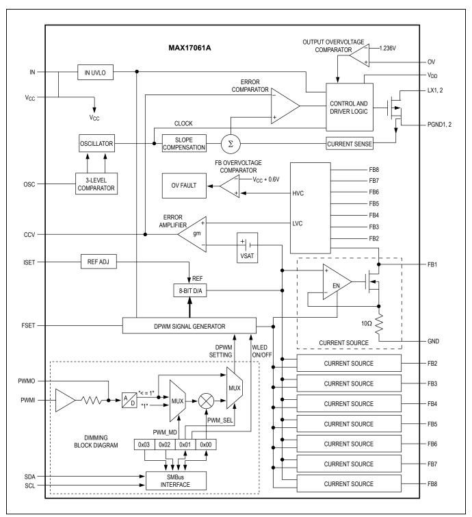
Figure 2. Control Circuit Block Diagram
