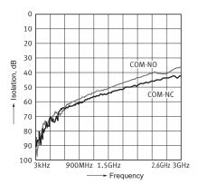
1-(2). High frequency characteristics (Impedance  $75\Omega)$  (Standard PC board terminal)
