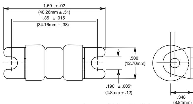
\*Recommend #8 Slotted Hex Washer Head Machine Screw for mounting
