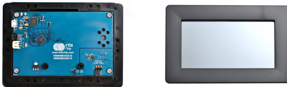
Figure 3-2 - VM800BU module profile 4.3" display version
