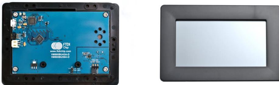
Figure 3-2 - VM800BU module profile 4.3" display version
