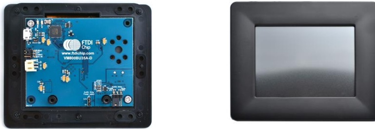
Figure 3-1 - VM800BU module profile 3.5" display version
