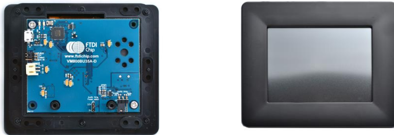
Figure 3-1 - VM800BU module profile 3.5" display version
