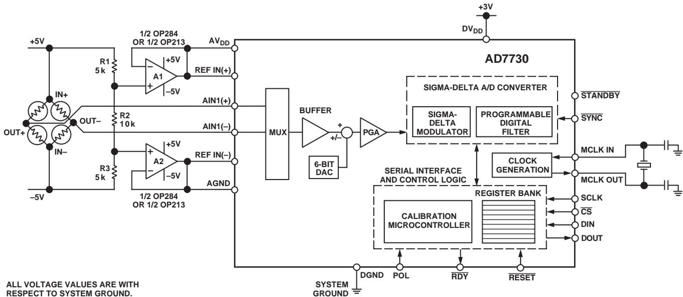
Figure 25. AD7730 with Bipolar Excitation of the Bridge
