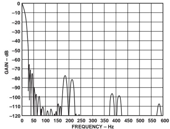
Figure 14. Expanded Full Frequency Response of AD7730 (Second Stage Filter as Normal FIR, Chop Disabled)
