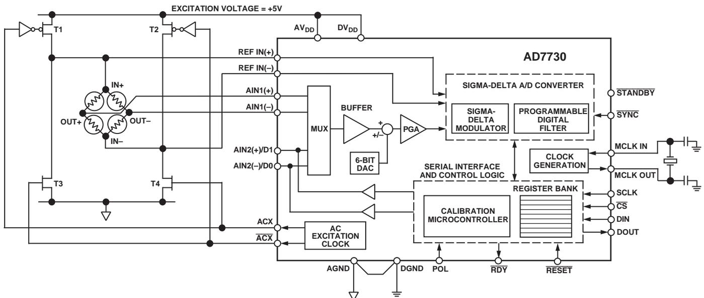
Figure 24. Typical Connections for AC-Excited Bridge Application
