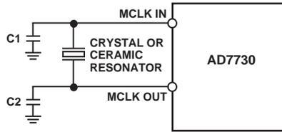
Figure 17. Crystal/Resonator Connections
