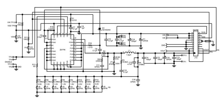
Schematic of MIC261203-ZA Evaluation Board (J11, R13, R15 are for testing purposes)
