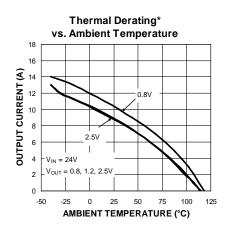
**Die Temperature\***: The temperature measurement was taken at the hottest point on the MIC261203-ZA while it was case mounted on a 5in<sup>2</sup> 4-layer, 0.62", FR-4 PCB, with 2oz finish copper weight per layer. See the "Thermal Measurements" section for more details. Actual results will depend on the size of the PCB, ambient temperature, and proximity to other heat emitting components.
