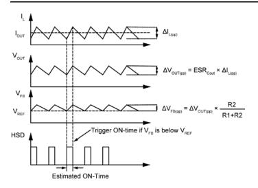
Figure 1. MIC261203-ZA Control Loop Timing
