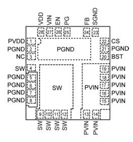
28-Pin 5mm × 6mm QFN (JL) (Top View)
