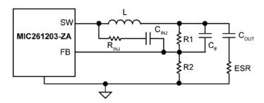
Figure 6. Invisible Ripple at FB
