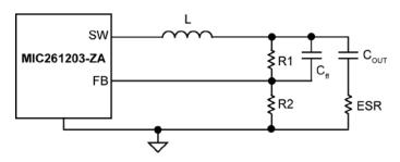
Figure 5. Inadequate Ripple at FB
