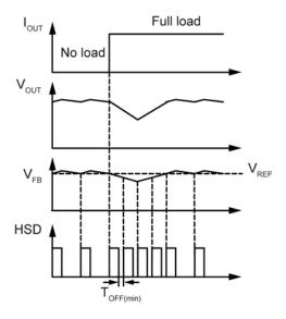
Figure 2. MIC261203-ZA Load Transient Response
