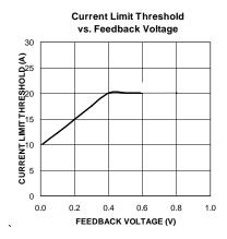
Figure 3. MIC261203-ZA Current-Limit Foldback Characteristic
