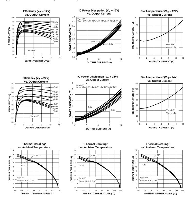
**Die Temperature\***: The temperature measurement was taken at the hottest point on the MIC261203-ZA while it was case mounted on a 5in<sup>2</sup> 4-layer, 0.62", FR-4 PCB, with 2oz finish copper weight per layer. See the "Thermal Measurements" section for more details. Actual results will depend on the size of the PCB, ambient temperature, and proximity to other heat emitting components.
