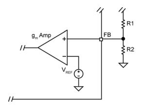
Figure 7. Voltage-Divider Configuration
