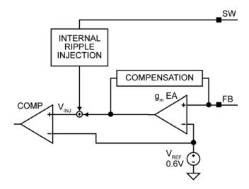
Figure 8. Internal Ripple Injection
