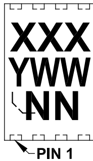
8-Lead TDFN (2x3x0.75 mm)
