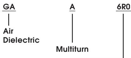
**Maximum Rated Capacitance —** expressed in pF by three digits. The first two are significant figures; the last specifies the number of zeros that follow. The letter R indicates a decimal point.
