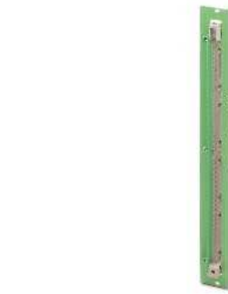
Converter for Siemens SIMATIC® S5-115 to 50-pos. FLK strip.
