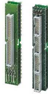
Front adapter for SIMATIC® S7-300, I/O cards with max. 32 channels
