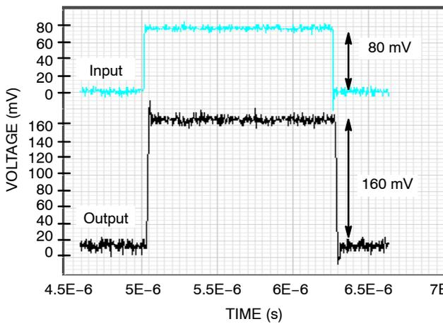
Figure 8. Small Signal Step Response
