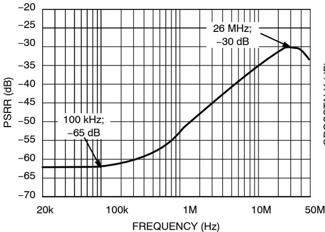
Figure 6. PSRR vs. Frequency (No Bypass Capacitor)
