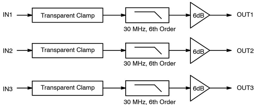
Figure 1. Block Diagram
