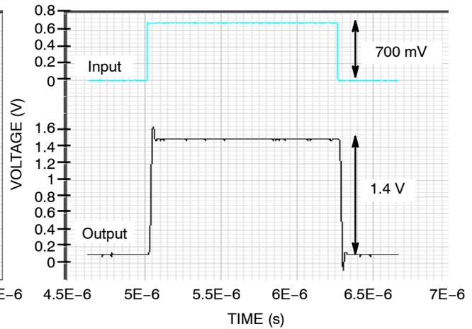
Figure 9. Large Signal Step Response
