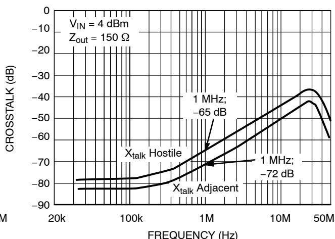
Figure 7. Crosstalk vs. Frequency, CH2/CH3
