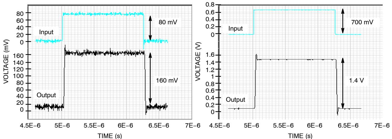
**Figure 8. Small Signal Step Response**
