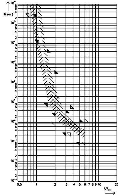
23 A - 150 A: FI = 1.25 (max. operating current:  $0.8 \times I_{rat}$  at  $23^\circ\text{C}$ )
