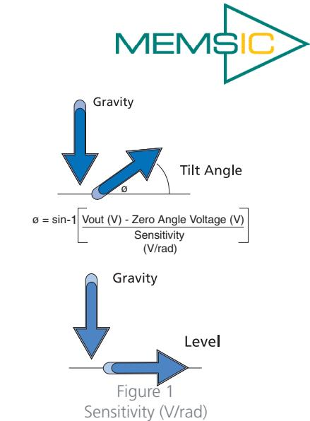
For angles less than 20°, the sine function can be approximated by a linear relationship between the  $V_{out}$  and the tilt angle in degrees. Thus the simplified equation for small angle in degrees is:
