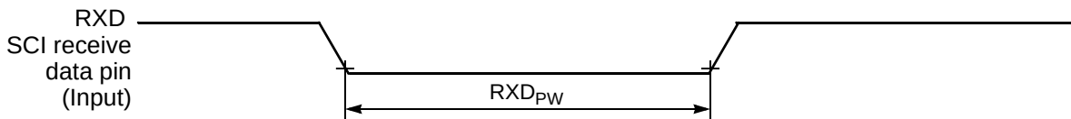
Figure 10-16 RXD Pulse Width
